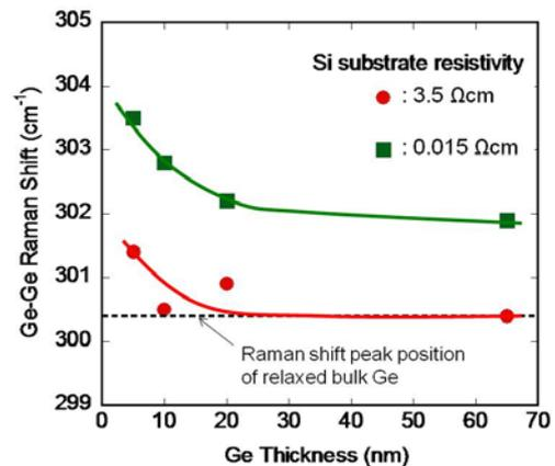
Fig. 3 Ge-Ge Raman shift peak positions, as function of Ge thickness, obtained from samples after Ge growths by 5, 10, 20 and 65 nm on 3.5 and 0.015  $\Omega\text{cm}$  Si substrates.
