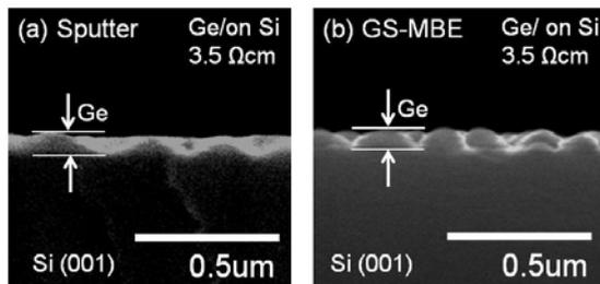
Fig. 1 Typical cross sectional SEM images obtained from Ge layers on Si formed by (a) sputter and (b) GS-MBE.
