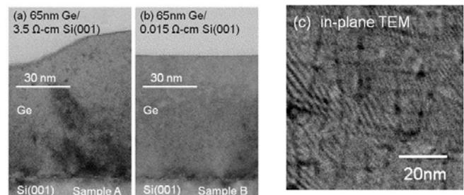
Fig. 4 TEM images obtained from Ge layers on (a) 3.5  $\Omega\text{cm}$  and (b) 0.015  $\Omega\text{cm}$  Si substrates and (c) in-plane TEM image of interface of Ge and Si 0.015  $\Omega\text{cm}$  Si substrate.
