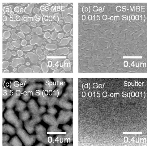
Fig. 2 Typical SEM images obtained from Ge layers formed by GS-MBE on (a) 3.5 and (b) 0.015  $\Omega\text{cm}$  Si, and formed by Sputter on (c) 3.5 and (d) 0.015  $\Omega\text{cm}$  Si.
