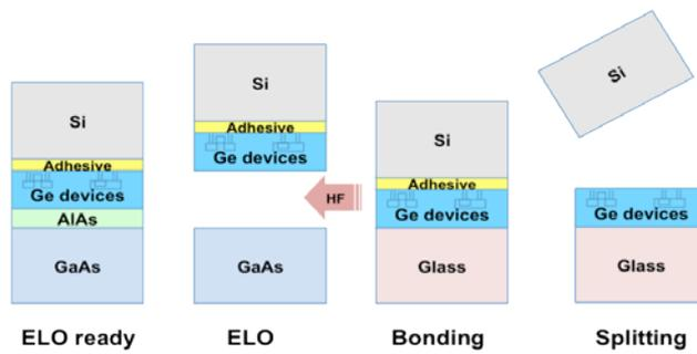
Figure 6. The process flow of Ge device layer transfer with ELO technique.
