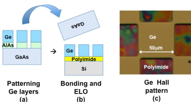
Figure 5. The schematic flow of the patterned Ge layer ELO process in device size ( $< 100 \times 100 \mu\text{m}^2$ ) ((a) and (b)). The photograph of the transferred Ge Hall pattern on Si with polyimide as an adhesive (c).
