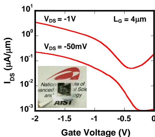
Figure 7.  $I_{DS}-V_G$  characteristics of Ge pMOSFET on glass ( $L_G = 4 \mu\text{m}$ ). The inset is the photograph of Ge device layer on glass including pMOSFETs, diodes, resistors, etc.
