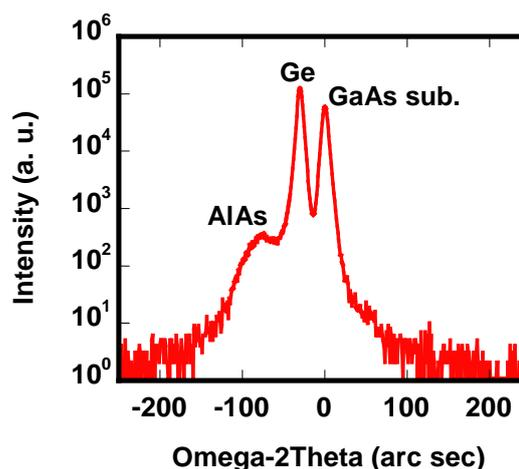
Figure 3. The measured XRD rocking curve from (004) refraction of the epitaxially grown Ge/AlAs layers on GaAs substrate.
