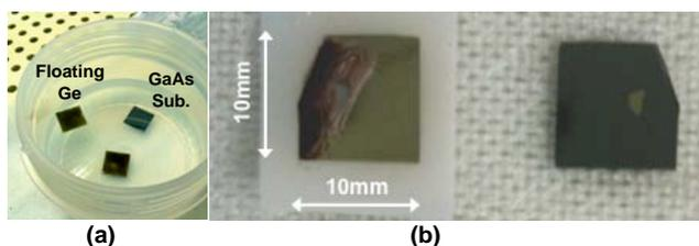
Figure 4. The photographs of (a) the floating Ge layer and GaAs donor substrate in HF solution and (b) the ELO Ge layer with die-level size ( $10 \times 10 \text{ mm}^2$ ) on the flexible plastic sheet with adhesive (left) and initial GaAs donor substrate (right).
