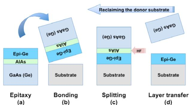
Figure 1. A schematic flow of the epitaxial lift-off (ELO) process of Ge layer. (a) Epitaxial Ge layer on GaAs (Ge) substrates with AlAs sacrificial layer. (b) Bonding with an arbitrary host substrate (c) Splitting at AlAs layer with HF solvent and (d) Epitaxial Ge layer transferred on host substrates.
