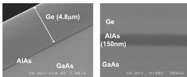
Figure 2. SEM images of epitaxial Ge/AlAs/GaAs heterostructure. The thicknesses of epitaxial Ge layer and AlAs sacrificial layer are 4.8 $\mu\text{m}$  and 150nm, respectively.
