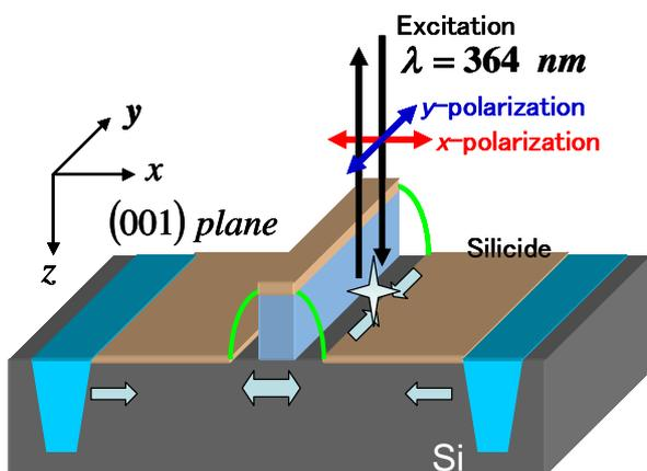
Fig. 1 Top down UV Raman measurement of Si-MOSFET structure.
