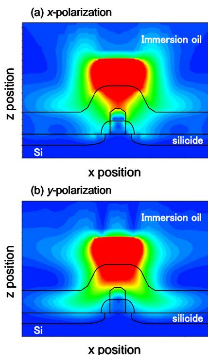
Fig. 3. 2D distribution of the light intensity calculated with the FDTD simulations for the light sources of (a) x-polarization and (b) y-polarization.
