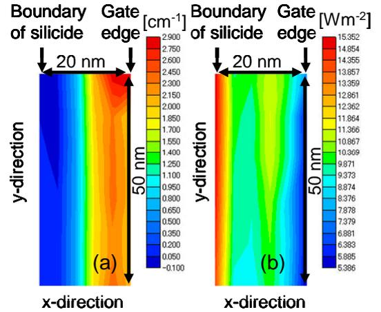
Fig. 5. 2D distribution of (a) Raman shift and (b) simulated light intensity in the offset spacer region. Right side: gate edge. Left side: boundary of silicide.
