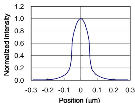
Fig. 2. Light intensity distribution at  $0.07 \mu\text{m}$  above the top of the stress liner.
