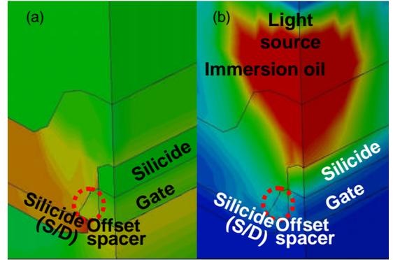
Fig. 4. 3D distribution of (a) Stress tensor  $\sigma_{xx}$  and (b) simulated light intensity of Si-MOSFET.
