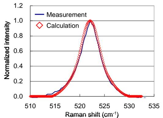
Fig. 6. Comparison of Raman spectra by calculation and measurement.
