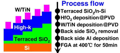
Fig. 1 Schematic diagram of MOS capacitors with a structure of W/TiN/HfO<sub>2</sub>/terraced-SiO<sub>2</sub>/Si and the process flow.
