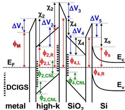
Fig. 2 Schematic diagram of energy band alignment of the MOS device with metal/high-k/SiO<sub>2</sub>/Si stack.
