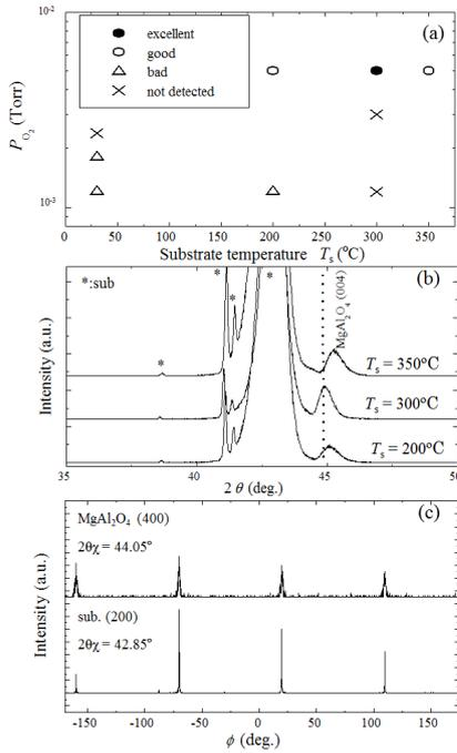
Fig. 1. (a) Film growth conditions and film crystallinity mapped in temperature versus  $P_{O_2}$  diagram. (b) XRD patterns for the films grown at 200, 300 and  $350^\circ\text{C}$ . (c) In-plane  $\phi$  scans for the  $\text{MgAl}_2\text{O}_4$  film grown at  $350^\circ\text{C}$  on MgO substrate.
