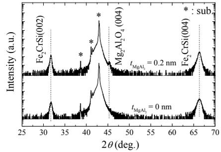
Fig. 2. XRD patterns of the multilayers with the thicknesses of  $t_{\text{MgAl}_2} = 0, 0.2$  nm.
