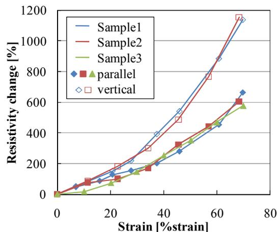
Fig.2 Changes of the resistance of the MWCNT-dispersed resin both parallel and perpendicular to the direction of the applied uni-axial strain
