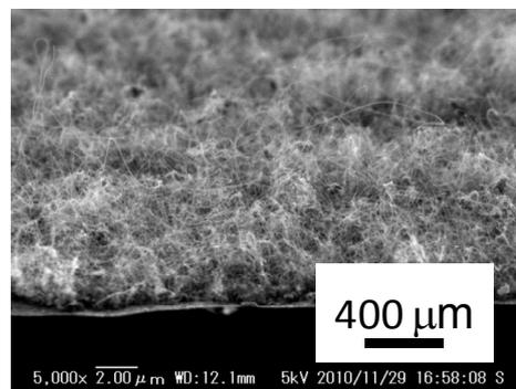
(b) MWCNTs grown on the 15-nm thick iron layer
