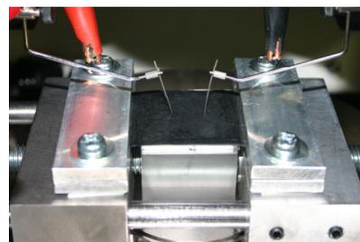
Fig. 1 Measurement of the change of resistance of a MWCNTs-dispersed resin under tensile strain
