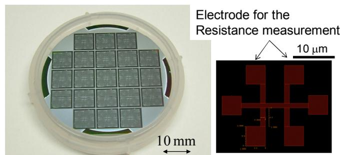
Fig. 4 Outlook of a Si wafer on which two-dimensional strain sensors using MWCNTs was formed
