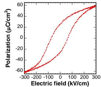
Fig. 1 Polarization-Electric field loop of PZT gate film.
