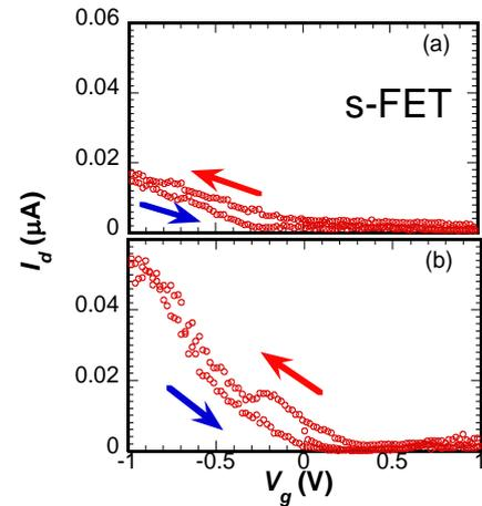
Fig. 5  $I_d$ - $V_g$  hysteresis characteristics (s-FET) (a) Before, (b) after dropping ionic liquid
