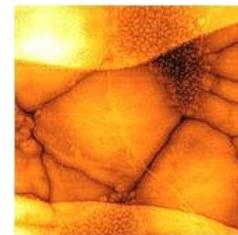
Fig. 3 AFM image of CNT channel taken through the ionic liquid covering the channel. The gap between source and drain electrodes is  $\sim 1 \mu\text{m}$ .
