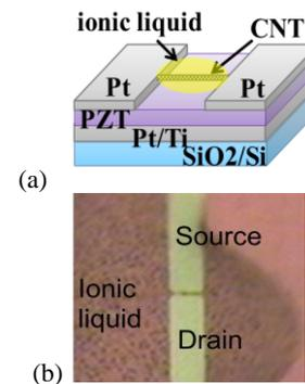
Fig. 2 (a) Schematic device structure and (b) optical microscopy image of FET channel covered with ionic liquid.
