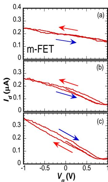
Fig. 4  $I_d$ - $V_g$  hysteresis characteristics (m-FET) (a) before, (b) just after dropping ionic liquid, (c) three days after dropping ionic liquid
