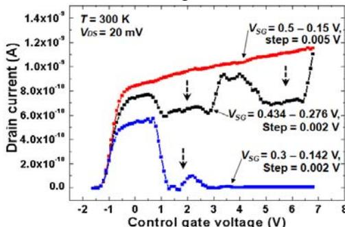
**Fig. 6.** Transfer characteristics of the fabricated SET with recessed channel structure with different side gate biases and bias steps in the same device at room temperature.
