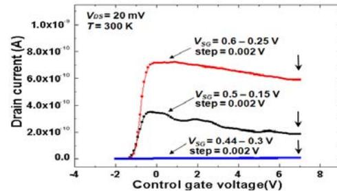
**Fig. 5.** Transfer characteristics of the fabricated device at room temperature. The drain current of the fabricated device is decreased when the control gate is increased.
