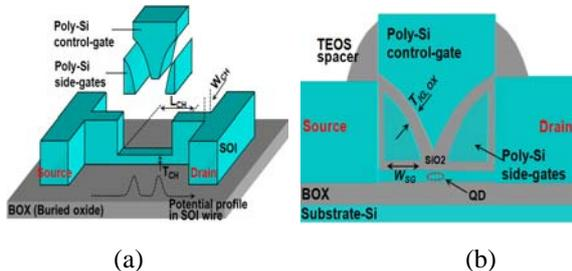
**Fig. 1.** Schematic three-dimensional layout of the proposed device having recessed channel structure (a) and oxide sidewall spacers around the control gate and potential profile along the channel by side gate bias (b).
