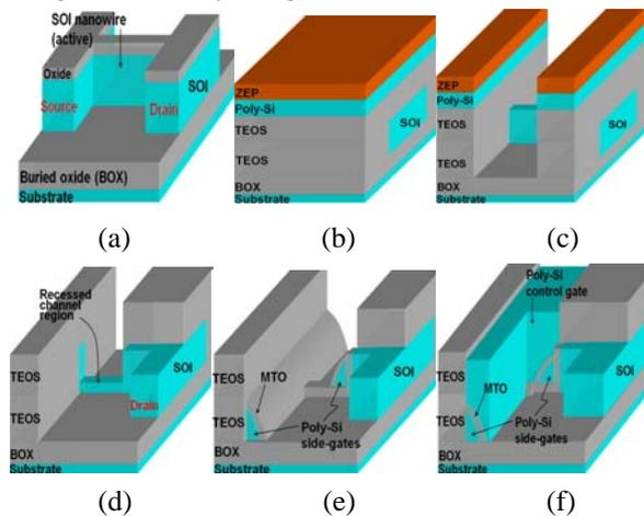
**Fig. 2.** Schematics of the process sequence of the nanowire patterning methods using the mix-and-match and proposed fabrication process flows of the sidewall patterning process.
