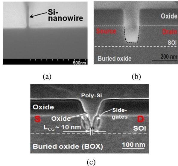
**Fig. 3.** (a) Cross-sectional SEM images of a test wafer for Si nanowire, (b) recessed channel structure of device, and (c) control gate formation.
