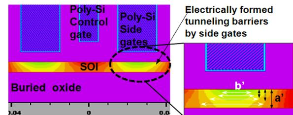
**Fig. 4.** Cross-sectional view along the channel region of the proposed device. Electrically potential distribution of the side gate bias when side gates are increased from 0.1 to 0.5 V.
