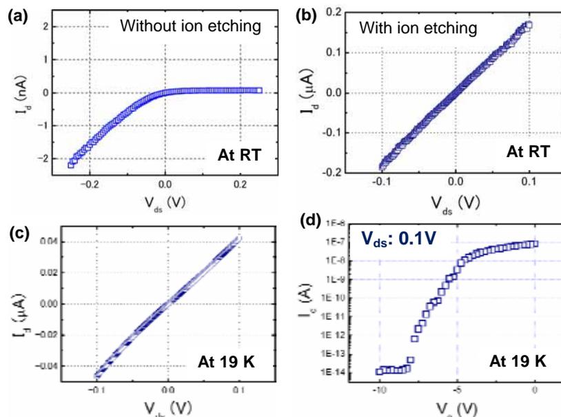
Fig. 3 Typical  $I_d$ - $V_d$  characteristics of InP NW-FET devices. (a) Without and (b) with Ar ion sputtering at RT. Typical (c)  $I_d$ - $V_d$  and (d)  $I_d$ - $V_g$  characteristics of the device with the sputtering process at 19 K.
