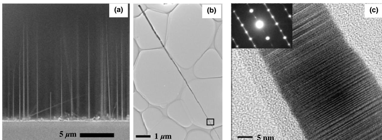
Fig. 1 (a) Cross-sectional SEM image of InP NWs epitaxially grown on a InP (111) substrate. (b) TEM image of a InP NW dispersed on a copper grid. (c) The HRTEM image of the rectangular region near the NW tip drawn in (b). The inset in (c) is the SED pattern, indicating the NW is dominated by the wurtzite structure with the  $\langle 0002 \rangle$  growth direction.
