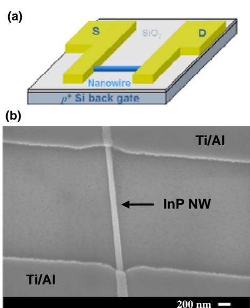
Fig. 2 (a) Schematic diagram and (b) SEM image of a FET device with an InP NW channel on a  $\text{SiO}_2/\text{Si}$  substrate.
