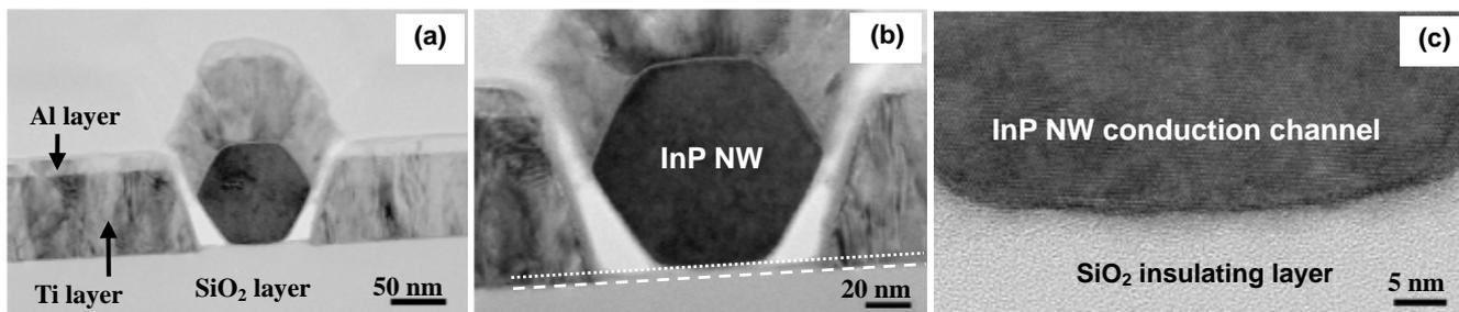
Fig. 4 (a) and (b) Cross-sectional TEM images of InP NW-FET devices with the Ar ion sputtering step. The dotted (dashed) line indicates the interfaces between the NW and the  $\text{SiO}_2$  layer (between the electrodes and the  $\text{SiO}_2$  layer). (c) HRTEM image of the interface between the InP NW and the underlying  $\text{SiO}_2$  layer.
