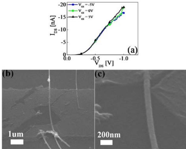
Fig. 3 (a)  $I_{DS}$ - $V_{DS}$  measured at  $V_{GS}$  values from  $-5$  V to  $5$  V. (b) and (c) SEM images of the first fabricated core-shell SiNW transistor ; broken graphene.
