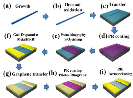
Fig. 1 Schematic process sequence of the graphene gated SiO<sub>2</sub> core-shell SiNW FETs.
