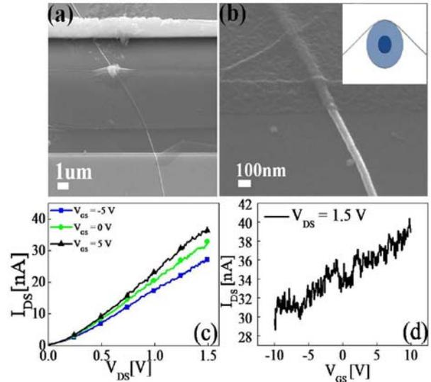
Fig. 5 (a) and (b) SEM images of the third fabricated core-shell SiNW transistor. (inset) Schematic showing the coverage of the graphene gate. (c)  $I_{DS}$ - $V_{DS}$  measured at  $V_{GS}$  values from  $-5$  V to  $5$  V. (d)  $I_{DS}$ - $V_{GS}$  at  $V_{DS} = 1.5$  V.
