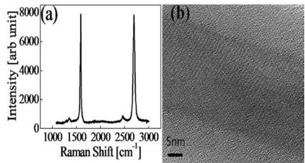
Fig. 2 (a) Raman spectrum of the CVD synthesized graphene. (b) TEM image of the SiO<sub>2</sub> core-shell silicon nanowire
