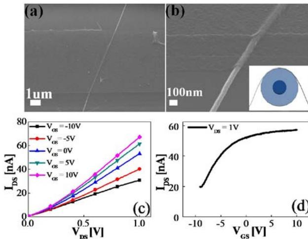
Fig. 4 (a) and (b) SEM images of the second fabricated core-shell SiNW transistor. (inset) Schematic showing the coverage of the graphene gate. (c)  $I_{DS}$ - $V_{DS}$  measured at  $V_{GS}$  values from  $-10$  V to  $10$  V. (d)  $I_{DS}$ - $V_{GS}$  at  $V_{DS} = 1$  V.
