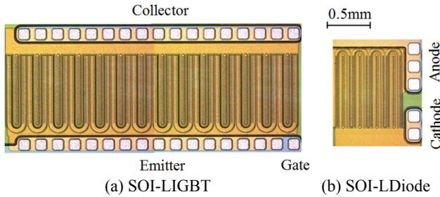
Fig. 1 Photos of the fabricated SOI-LIGBT and LDiode chips.
