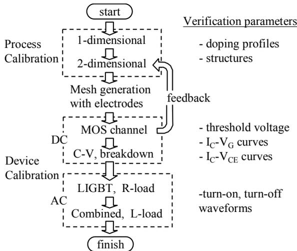
Fig. 3 Conceptual flowchart of the TCAD calibration methodology for SOI-LIGBT & LDiode system.
