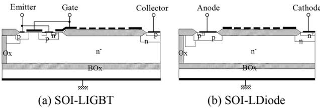
Fig. 2 Schematic cross-sectional device structures.
