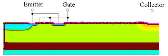
Fig. 4 SOI-LIGBT structure after process calibration.
