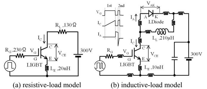
(a) resistive-load model (b) inductive-load model
