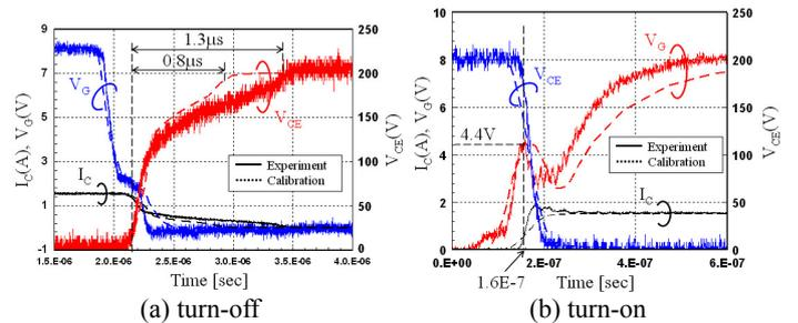
Fig. 7 Simulated switching waveforms after AC calibration of SOI-LIGBT using resistive-load model compared with measured waveforms. Dashed lines: simulation, Solid lines: experiment.
