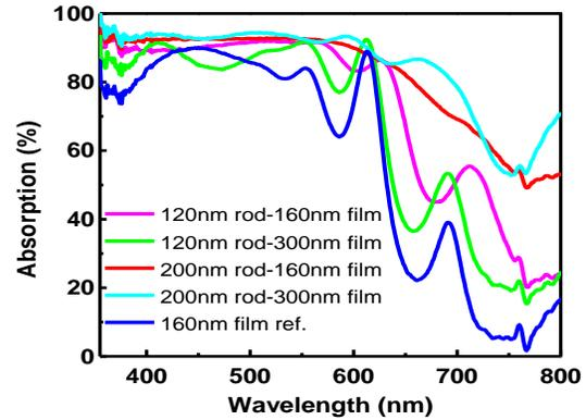
Fig.4 The absorption of active layers of amorphous thin film solar cell with ITO patterned electrode.
