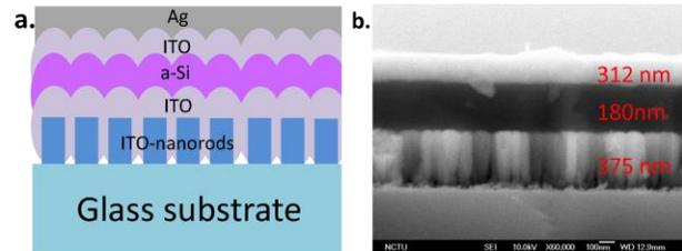
Fig. 1 (a)The schematic of amorphous silicon thin film solar cell utilizing the ITO nano-rods patterned electrode. (b) Scanning electron microscopic (SEM) image of the amorphous silicon thin film solar cell
