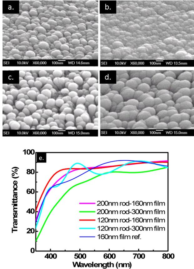
Fig. 3 SEM image of ITO sub wavelength structure and its transmittance. (a) 120 nm rod with 160 nm film. (b) 120 nm rod with 300 nm film. (c) 200 nm rod with 160 nm film. (d) 200 nm rod with 300 nm film. (e) The transmittance of structures
