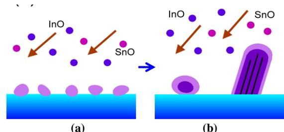
Fig.2 growth mechanism of ITO whiskers breaks into three main step: (a) the nucleation, (b) rod growth.
