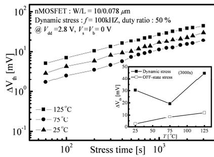
Fig. 4.  $\Delta V_{th}$  versus dynamic stress time at different  $T$ 's. The inset shows  $T$  dependency of  $\Delta V_{th}$  for dynamic and OFF-state stresses.
