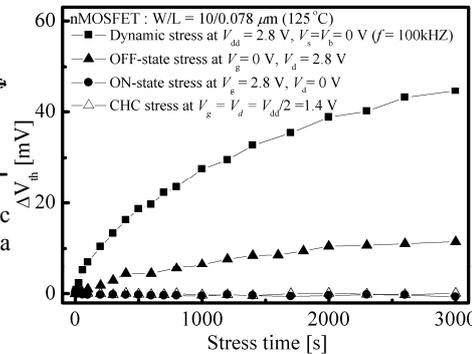
Fig. 2.  $\Delta V_{th}$  versus stress time for nMOSFETs subjected to various stress modes at  $T = 125^\circ\text{C}$ .
