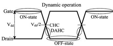
Fig. 1. Schematic of the dynamic stress condition of nMOSFET in a CMOS inverter circuit.
