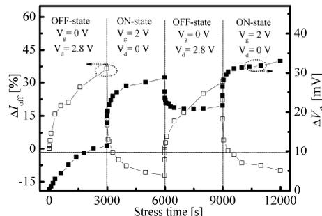
Fig. 5.  $\Delta V_{th}$  and  $\Delta I_{off}$  versus stress time alternating between OFF and ON-states.
