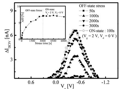
Fig. 6.  $\Delta I_{DCIV}$  versus  $V_g$  after OFF-state stress. The inset shows the corresponding  $\Delta SS$  behavior.
