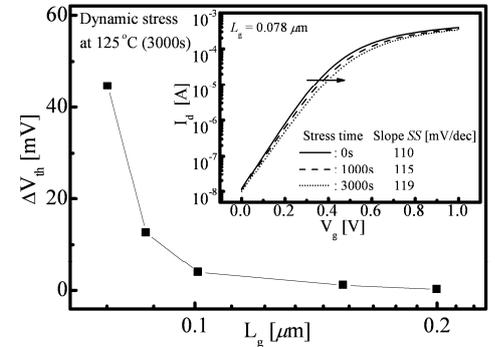
Fig. 3.  $L_g$  dependence of the dynamic stress. The inset shows shifts of  $I_d$ - $V_g$  curves for  $L_g = 0.078 \mu\text{m}$  measured at  $V_d = 0.05 \text{ V}$ .
