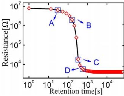
Fig.4 Resistance evolution with the Retention time for the cell in the initial amorphous state. (T=200°C)
