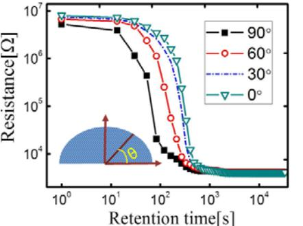
Fig.12 Simulated R-t curves with the initial same amount grains at different  $\theta$  angles to the horizontal axis.
