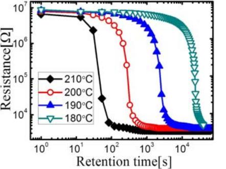
Fig.9 Simulated R-t curves at the temperature of 210°C, 200°C, 190°C and 180°C in the retention process.
