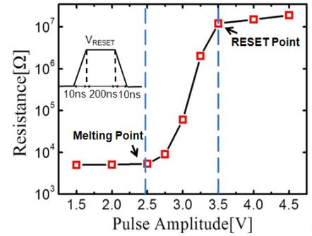
Fig.3 Resistance evolution with the increasing RESET Pulse voltage for the cell in the initial crystalline state.
