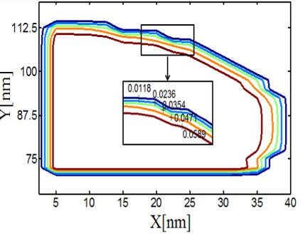
Fig.8 Inner nucleation probability in the phase change area. (point B in Fig.5)
