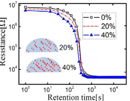
Fig.11 Simulated R-t curves with different initial crystallization grain proportion (0%, 20% and 40%) with random distribution.
