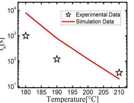
Fig.10 Simulated  $t_h$ -T curves for the different retention temperatures. The experimental data [7] is also shown.
