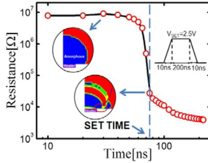
Fig.2 Resistance evolution with variable SET time for the cell in the initial amorphous state.
