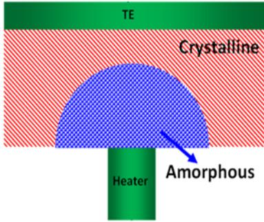
Fig.1 Schematic of a PCM cell simulated in this research.
