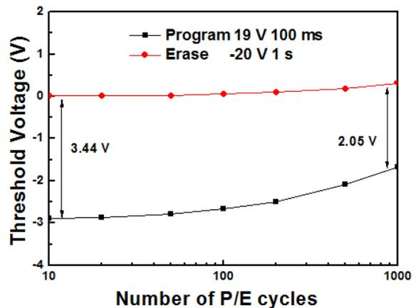
Fig. 5. Endurance characteristics of TBE-TFT memory device on glass substrate. The device was programmed and erased by applying +19 V at 100 ms and -20 V at 1 s, respectively.
