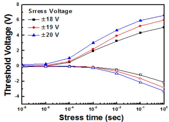
Fig. 3. Programming and erasing characteristics of a TBE-TFT memory device on glass substrate.
