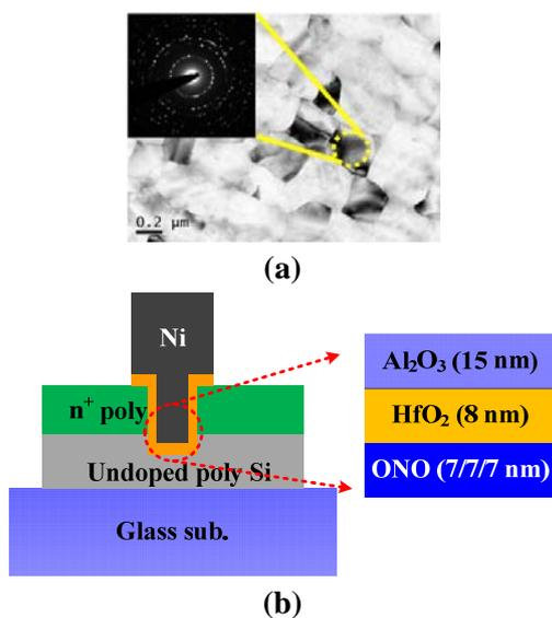
Fig. 1. (a) TEM image of microcrystal-line silicon films formed on glass using ELA method and electron beam diffraction patterns within the grain. (b) Recess-channel TBE-FET memory device on glass substrate and tunnel, trap and blocking layers, respectively.
