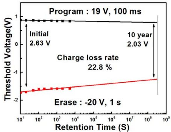
Fig. 4. Charge retention characteristics of TBE-TFT memory device on glass substrate. The device was programmed and erased by applying +19 V at 100 ms and -20 V at 1 s, respectively.
