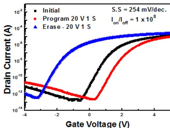
Fig. 2. Transfer and P/E characteristics of a TBE-TFT memory device on glass substrate. The device was programmed and erased by applying +20 and -20 V, respectively.
