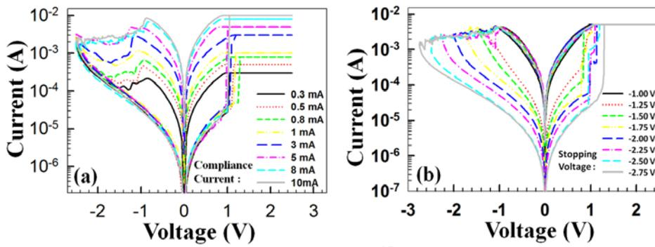
Fig. 1 Bipolar switching behaviors of TiN/SiO<sub>2</sub>/FeO<sub>x</sub>/Fe structure under (a) a series of compliance current in set process fixed stopped voltage and (b) a series of stopped voltage in reset process fixed compliance current.
