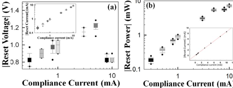
Fig. 2 Statistics plots of (a) reset voltage and current (inset) as a function of compliance current and (b) reset power as a function of compliance current. The red dash fitting line in the inset of (b) shows a linear dependence between two currents.
