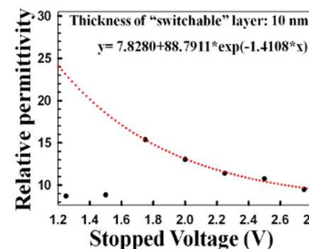
Fig. 5 (a) Linear fitting results for the TiN/SiO<sub>2</sub>/FeO<sub>x</sub>/Fe structure under a series of stopped voltage in the HRS region. (b) A plot of  $\ln(J/V)$  vs  $V^{1/2}$  under a series of stopped voltage in the HRS region. The linearity criterion of fitting curves is over 99%.
