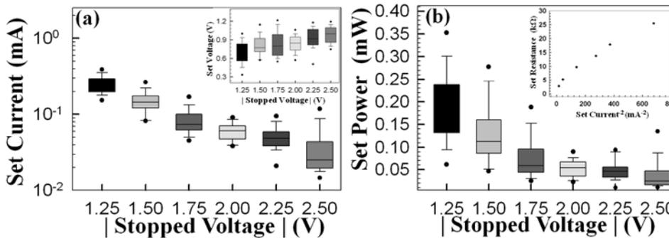
Fig. 3 Statistics plots of (a) set current and voltage (inset) as a function of stopped voltage and (b) set power as a function of stopped voltage. The inset shows the relation between  $R_{set}$  and  $I_{set}^{-2}$  under a series of stopped voltage.
