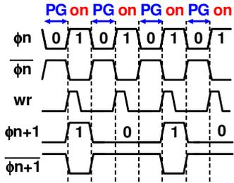
Fig. 3 The operating waveforms of the proposed counter.
