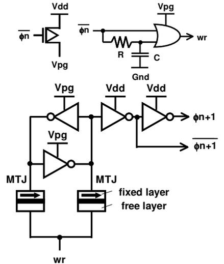
Fig. 2 The proposed nonvolatile counter unit.
