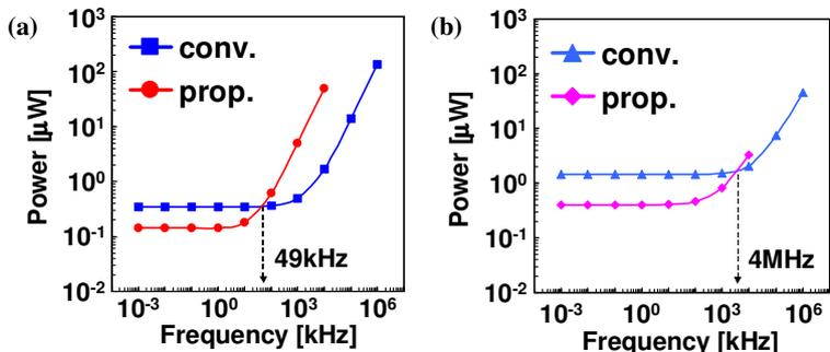
Fig. 8 The comparison of the power of the 32-bit counter using the proposed units and that using the conventional units for (a) 45nm node and (b) 16nm node.
