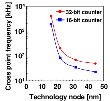
Fig. 9 The trend of the cross point frequencies for the 16-bit and the 32-bit counters from 45nm node to 16nm node.
