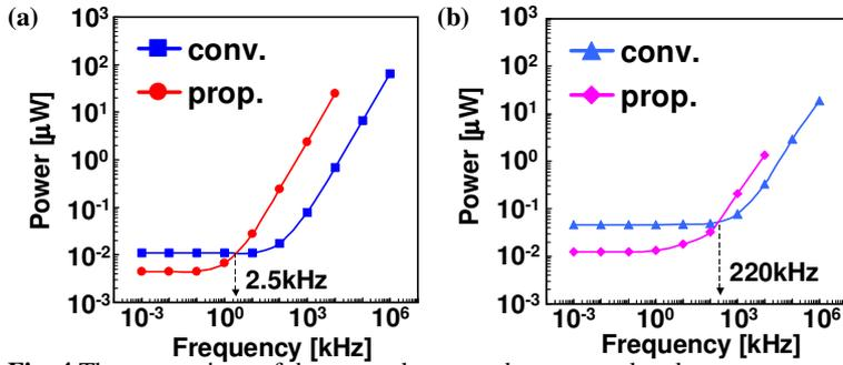
Fig. 4 The comparison of the power between the proposed and the conventional counter units for (a) 45nm node and (b) 16nm node.
