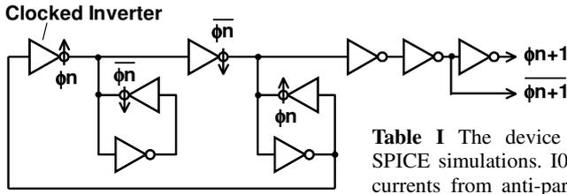
Fig. 1 The conventional counter unit.
