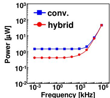
Fig. 11 The power comparison of the 32-bit counters between the conventional and the hybrid proposed.
