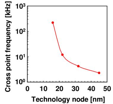
Fig. 5 The trend of the cross point frequencies for the counter units from 45nm node to 16nm node.
