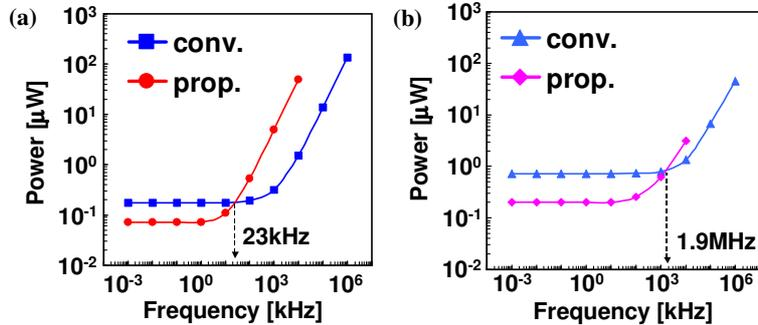
Fig. 7. The comparison of the power of the 16-bit counter using the proposed units and that using the conventional units for (a) 45nm node and (b) 16nm node.
