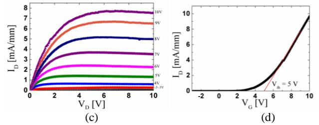
Fig. 5. ID-VD and ID-VG characteristics of (a),(b) trench-gate MOSFET and (c),(d) mesa-gate MOSFET after TMAH treatment.
