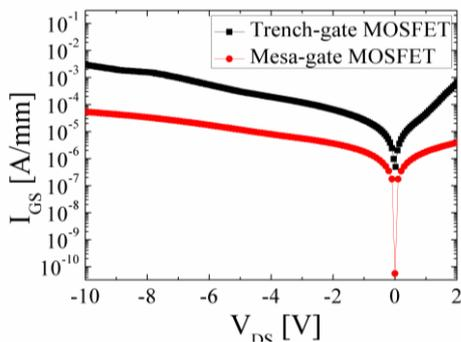
Fig. 3. The gate leakage current of trench-gate and mesa-gate MOSFET.
