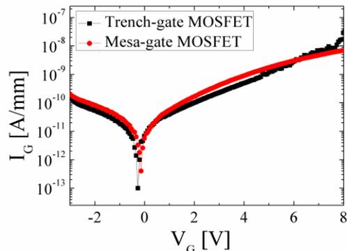
Fig. 6. The gate leakage current of trench-gate and mesa-gate MOSFET after TMAH treatment.
