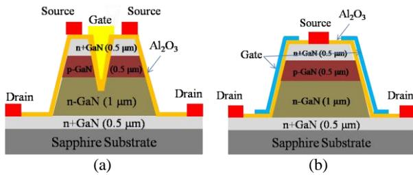
Fig. 1. Schematic of device structure for (a) trench-gate MOSFET and (b) mesa-gate MOSFET.
