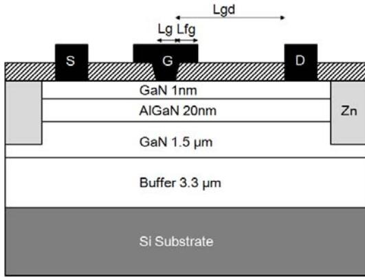
Fig. 1 Device structure of a high-voltage AlGaIn/GaN HEMT on a p-type Si substrate
