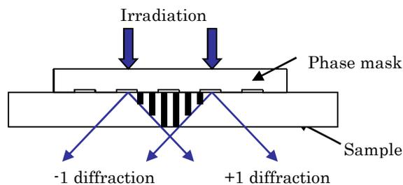
Fig. 2 Formation principle of the grating using a phase mask.
