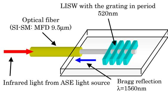
Fig. 3 Schema of the band-pass filter which consists of a LISW waveguide and the grating.
