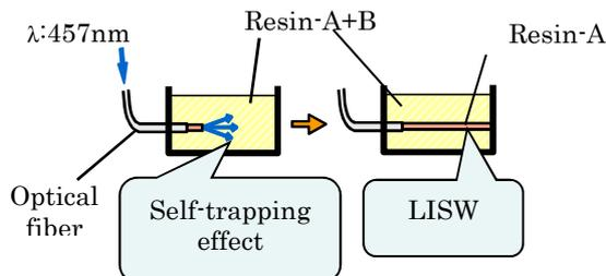
Fig. 1 Formation principle of the LISW waveguide.
