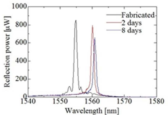
Fig. 6 Spectra of the filter function after just-fabricated, 2 days and 8 days, respectively. This graph shows the stability of fabricated filter.
