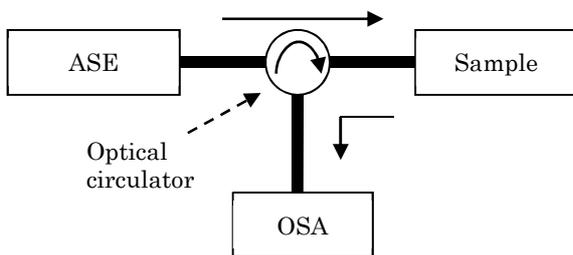
Fig. 4. Schema of the set up used for measuring the band-pass filter characteristics.
