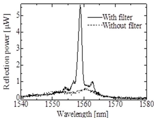
Fig. 5 Reflection spectra from the sample with/without the band-pass filter to a LISW waveguide.
