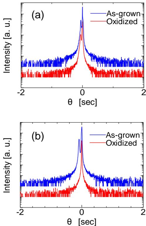
Fig. 2. XRD  $\theta$ - $2\theta$  scans for the  $\text{Al}_x\text{Ga}_{1-x}\text{As}$  samples of (a)  $x = 0.55$  and (b)  $0.86$  before and after oxidation.
