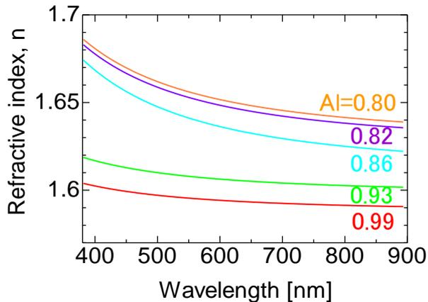
Fig. 3. Wavelength dispersions of the refractive index for the oxide layers investigated. The initial Al concentration were indicated in the figure.
