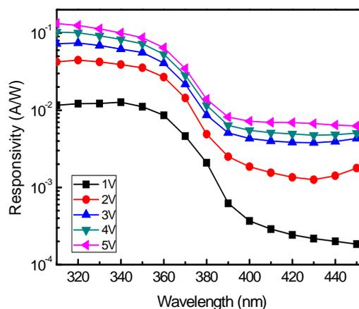
Fig. 3 Spectral responses measured from the GaN MIS PDs with a CsF current suppressing layer.
