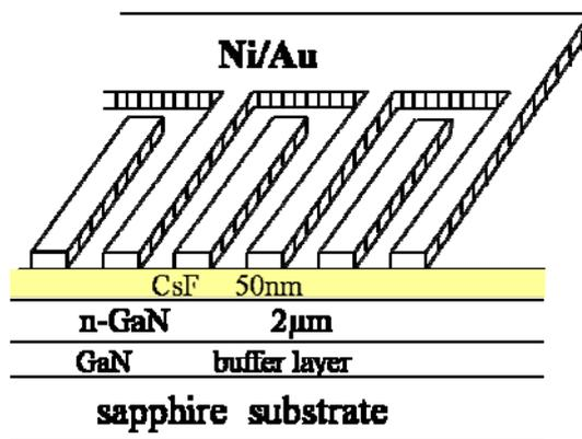
Fig. 1 The schematic structure of GaN MIS PDs with a CsF current suppressing layer
