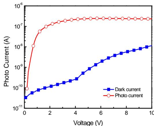
Fig. 2 I-V characteristics measured from the GaN MIS PDs with a CsF current suppressing layer at dark and under illumination.
