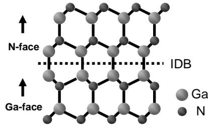
Fig. 2 Schematic of inversion domain boundary (IDB).
