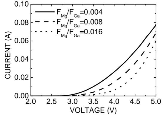
Fig. 4  $I$ - $V$  curves of samples for the flow ratio of p-type layer with 0.004, 0.008, and 0.016, respectively.
