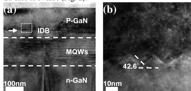
Fig. 1 (a) Cross-sectional TEM image of LED with 0.016 flow ratio. (b) High-magnification TEM image of pyramidal interface in *p*-layer.
