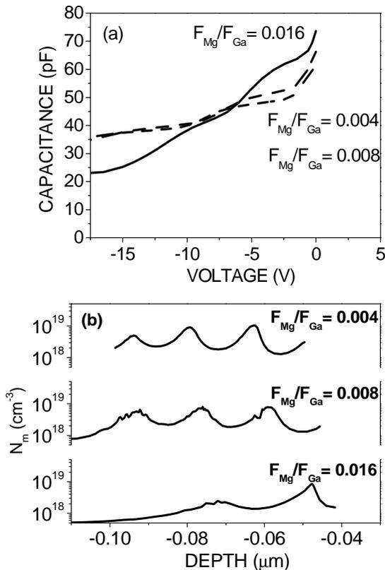
Fig. 3 (a)  $C$ - $V$  curves of samples for the flow ratio of p-type layer with 0.004, 0.008, and 0.016, respectively. (b) Depth profiles of the apparent carrier distribution obtained from (a).
