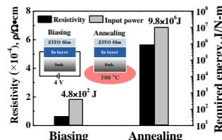
Figure 4 Schematic illustration for resistivity and required energy of ZITO/In film with different treatments.
