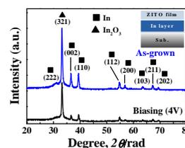
Figure 2 XRD patterns of un-biased ZITO/In sample and ZITO/In sample with biased of 4V.
