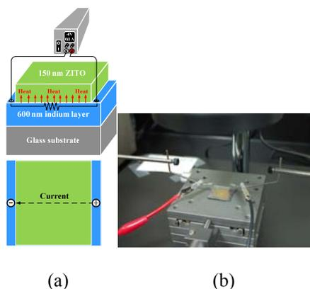
Figure 1 (a) The schematic illustration and (b) the photograph of bias-crystallized for ZITO film.
