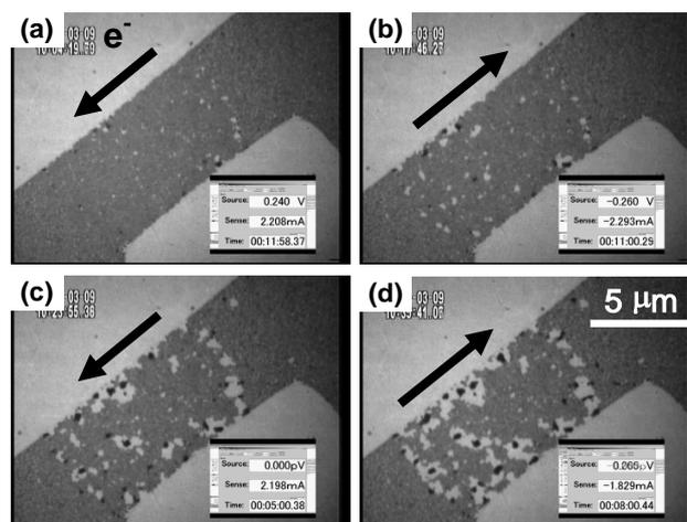
**Fig. 1** A series of TEM images of Au narrow wire during alternation of the current flow. The arrows indicate the flow of electron which is opposite to the current flow. TEM images (a) after the current flow along one direction, and (b) to (d) after repeat of the current alternation.
