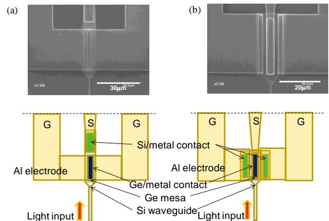
Fig. 2 SEM images and schematic diagrams of Si waveguide-integrated PIN Ge-PDs of (a) back-contact and (b) side-contact structures for Si and metal contact.
