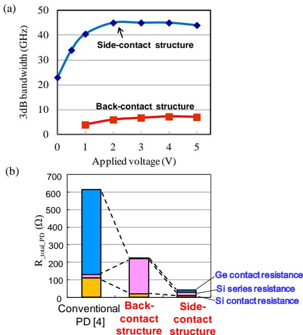
Fig. 4 (a) Dependence of 3dB bandwidth for PIN Ge-PDs of back-contact and side-contact structures on dc bias voltage. (b) Details of additional resistance for three different PIN Ge-PDs of conventional PD, back-contact, and side-contact structures.
