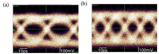
Fig. 5 Measured eye diagrams for the PIN Ge-PD of side-contact structure in case of (a) 25 Gbps at 0  $V_{\text{dc}}$  and (b) 40 Gbps at 3 $V_{\text{dc}}$  with 2<sup>15</sup>-1 PRBS.
