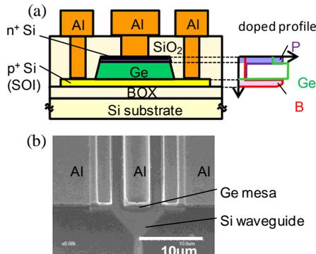
Fig. 1 (a) Schematic diagram and (b) SEM image of the Si waveguide integrated PIN Ge-PD.
