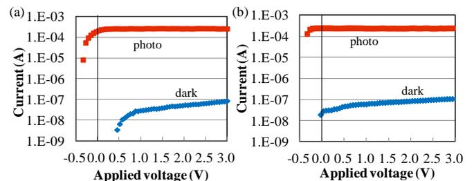
Fig. 3 Photoresponsivity of the fabricated PIN Ge-PD for (a) back-contact and (b) side-contact structures.
