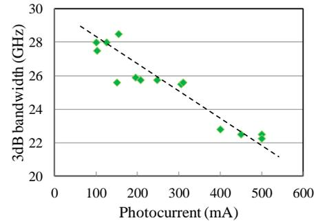
Fig. 6 Dependence of 3dB bandwidth for the PIN Ge-PD of side-contact structure on photocurrent.
