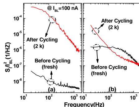
Fig. 2. Normalized noise power spectra corresponding to  $I_{BL}$  fluctuations in Fig. 1 (a)-(b) and (c)-(d).
