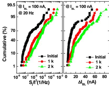
Fig. 3. Cumulative probability of noise power spectral densities at 20 Hz and  $\Delta I_{BL}$  with cycling stress. Here,  $I_{BL}$  is fixed at 100 nA.
