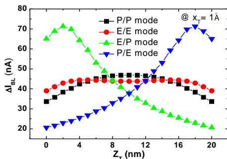
Fig. 5. Simulated  $\Delta I_{BL}$  with a trap position along the channel width ( $z_T$ ) as a parameter of the state (program or erase) of adjacent BL cells when the trap depth ( $x_T$ ) is 1 Å.
