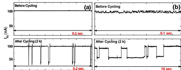
Fig. 1. Bit-line current fluctuation ( $\Delta I_{BL}$ ) in time domain before and after cycling stresses. (a)-(b) RTN is generated after 2k cycling. (c)-(d) Multi-level RTN is generated after 2k cycling.
