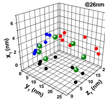
Fig. 6. Extracted  $x_T$ ,  $y_T$  and  $z_T$  of cycling stress induced traps in the tunneling oxide. Small symbols are trap position projected on each plane.
