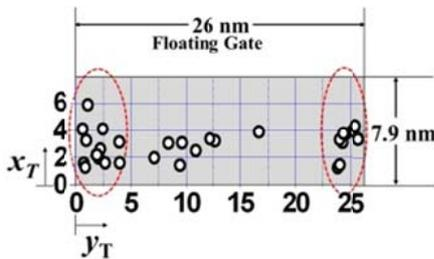
Fig. 4 Extracted vertical ( $x_T$ ) and lateral ( $y_T$ ) trap positions of process induced traps in the tunneling oxide.
