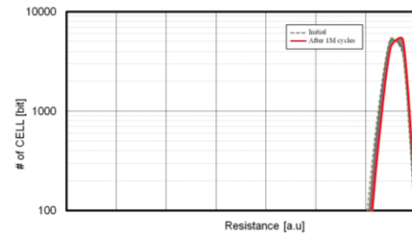
Fig. 7 Reset resistance distribution of the nearest cell according to the number of the programming cycles
