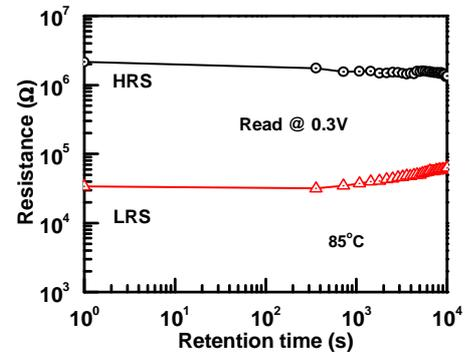
Fig. 13 Retention characteristics of fabricated cross point memory device at 85 °C. Both the memory states were maintained after 3 hours of testing.
