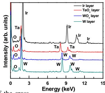
Fig. 2 EDX spectra of memory device. The presence of O peak in TaO<sub>x</sub> and WO<sub>x</sub> layers indicate formation of respective oxides.
