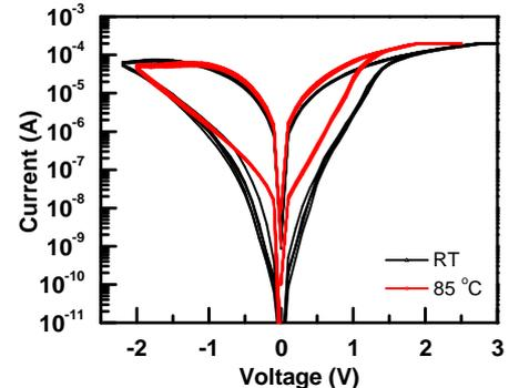
Fig. 10 Comparison of I-V curves at RT and 85 °C. The resistance of both HRS and LRS decrease at 85 °C.
