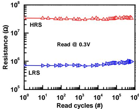
Fig. 11 Good read endurance of >6.5x10<sup>5</sup> cycles at read voltage of 0.3V is achieved with no obvious change in HRS and LRS.
