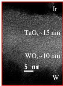
Fig. 1 HRTEM image of the cross point resistive memory device in a Ir/TaO<sub>x</sub>/W structure. The thickness of high-κTaO<sub>x</sub> film is 15 nm and device size is 4x4 μm<sup>2</sup>.
