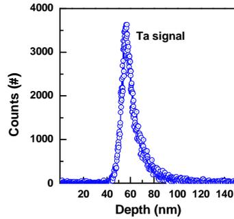
Fig. 3 Typical SIMS profile of TaO<sub>x</sub> film.
