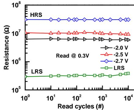
Fig. 9 Multilevel capability of memory device by limiting the reset voltage. Three data levels are obtained at reset voltage of -2.0, -2.5 and -2.7 V.
