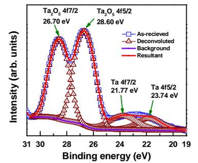
Fig. 4 XPS spectra of (a) TaO<sub>x</sub> layer. The peaks of Ta<sup>+5</sup> along with Ta<sup>0</sup> oxidation states in the XPS spectra confirm the formation of oxygen deficient tantalum oxide (TaO<sub>x</sub>) film
