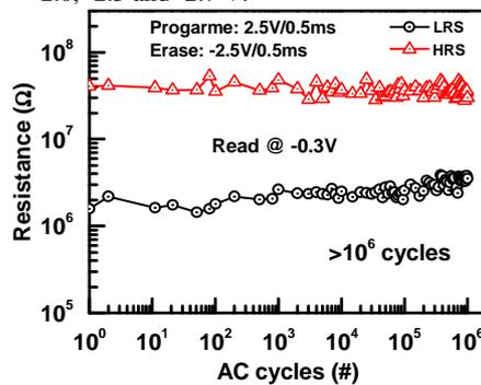
Fig. 12 Excellent pulse endurance of >10<sup>6</sup> P/E cycles with small pulse voltage of +/- 2.5 V is obtained. The device was live after 10<sup>6</sup> cycles indicating much higher endurance capability.
