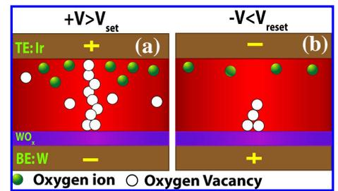
Fig. 7 Schematic representation of proposed switching mechanism based on filamentary model (a) low resistance state (LRS) occurs due to O<sub>2</sub> vacancy filament formation (b) high resistance state (HRS) obtained after filament rupture.
