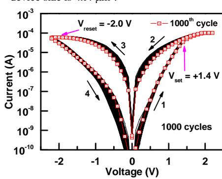
Fig. 5 Current-voltage (I-V) hysteresis characteristics of Ir/TaO<sub>x</sub>/W cross point memory device. Excellent reversible switching is achieved.
