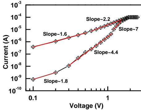
Fig. 6 Log-log plot of I-V curve of positive voltage region fitted linearly. Both LRS and HRS fitted to SCLC mechanism.
