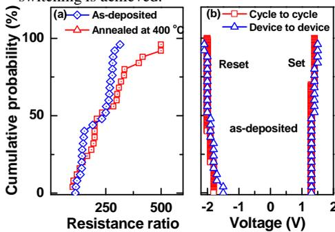
Fig. 8 Cumulative probability plot of (a) HRS/LRS of as-deposited and annealed samples and (b) set/reset voltage. Tight distribution is obtained.
