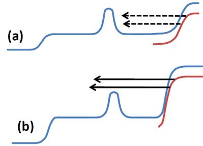
Fig. 7. Schematic energy band diagram to explain the threshold switching model. Injection from the substrate is assumed to take place from the valence band by band-to-band tunneling. Top figure represents the HRS and the bottom figure the LRS. The bistability observed during the TS loop can be explained by the existence of two field configurations.
