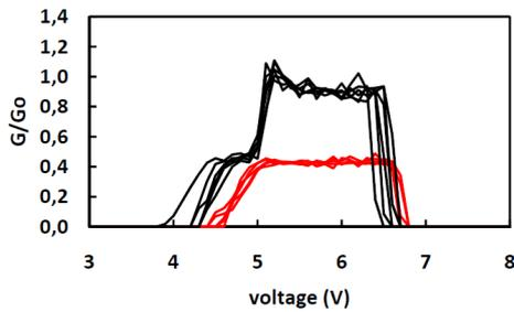
Fig. 5. Normalized conductance during the RESET cycle for a single level CF (red curves) and the two-level CF (black curves). Non-integer multiples of  $G_0$  are expected for quantum wires in the high bias regime.
