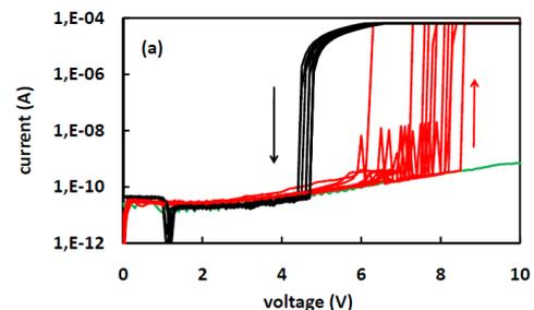
Fig.2 Experimental threshold switching loop. The High-Resistance State (HRS) is controlled by the background injection since the current fully coincides with that before forming (green curve). The SET transitions (red curves) occur in a wide range of voltages while the RESET voltage (black curves) distribution is narrower. In the conduction in the LRS is linear and the conductance is a fraction of the conductance quantum  $G_0=2e^2/h$ .
