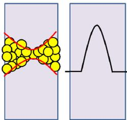
Fig. 6 Left figure: schematic representation of the CF structure (a conducting path made of "defects") with a constriction. Right figure: potential barrier associated to the position of bottom of the first quasi-1D subband in the CF.
