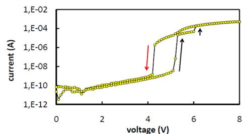
Fig.4 Two-level threshold switching loop. The existence of two sub-branches in the LRS strongly supports the quantum-wire model for the CF conduction. In the present case, the CF was wide enough to present two quantum subbands below the injecting Fermi level in the p-Si substrate
