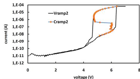
Fig. 3. Threshold switching loop measured with a current ramp (circles and blue line) and a voltage ramp (black line).
