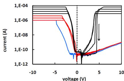
Fig.1 Electroforming by successive voltage ramps from 10V to -10V with current compliance increasing from 1μA to 64μA.
