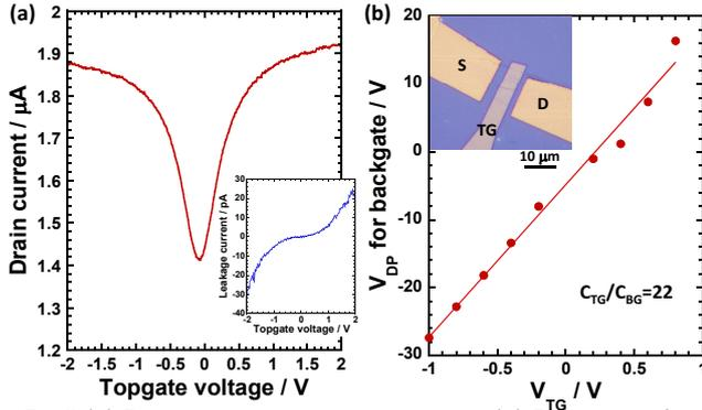
**Fig.2** (a) Drain current vs topgate voltage, (b) Dirac point for backgate sweep at different  $V_{TG}$ .
