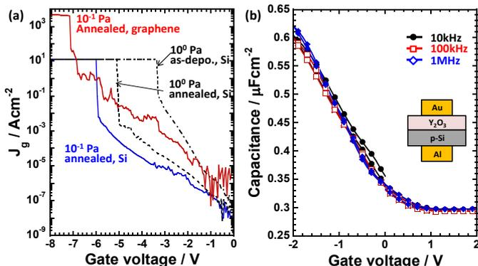
**Fig.1** (a) Leakage current of  $Y_2O_3$ , (b) bidirectional CV curve of MOS capacitor.
