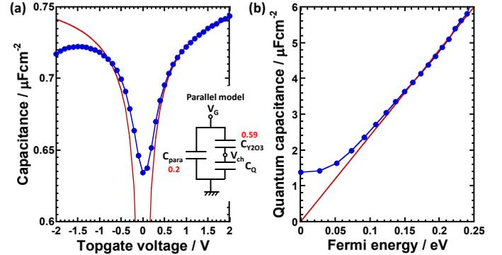
**Fig.3** (a) Total topgate capacitance vs  $V_{TG}$ , (b) Estimated  $C_Q$  with theoretically predicted  $C_Q$  (solid line).
