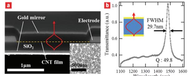
Fig. 2. (a) Cross section SEM image of gold mirror microcavity device. Inset: SEM image of CNT film. (b) Transmittance of the microcavity device. Inset: Schematic photonic mode profile.
