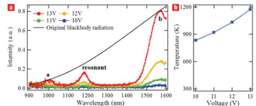
Fig.5. (a) Emission spectra from DBR device at 13 V (red), 12 V (yellow), 11 V (green), 10 V (blue). (Black line) Original blackbody radiation at 13 V = 1172.6 K. (b) CNT film temperature versus applied voltage.
