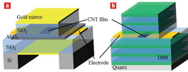
Fig. 1. 3D schematic pictures of the CNT film light emitter with microcavity: (a) Au metal mirror device and (b) distributed Bragg reflector device.
