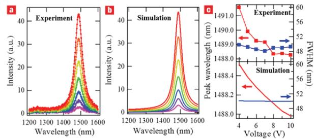
Fig.3. (a) Emission spectra from film CNT light emitter with gold mirror microcavity at seven biases  $V = 10$  V (red), 9 V (orange), 8 V (yellow), 7 V (green), 6 V (blue), 5 V (purple), 4 V (magenta). (b) Simulated emission spectra. (c) Peak wavelength and FWHM extracted from experimental and simulated emission spectra.
