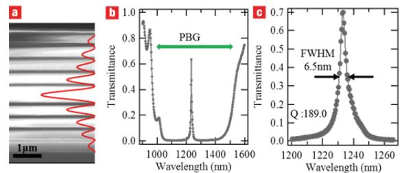
Fig.4. (a) Cross section SEM image of DBR device. (b) Transmittance of fabricated DBR. (c) Magnified resonant peak of transmittance.
