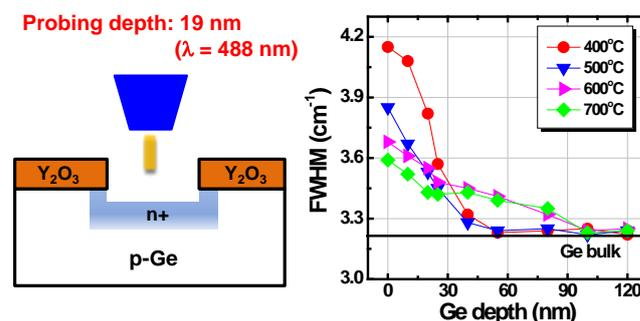
**Fig. 3** Ge depth profile of FWHM in phosphorus implanted region after dopant activation annealing. It is worth noting that laser wavelength of Raman spectroscopy is 488 nm and probing depth in Ge is around 19 nm.
