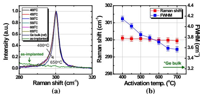
**Fig. 2** (a) Raman spectra for Ge wafers implanted with phosphorus as a function of dopant activation temperature. (b) Both position and full width at half maximum (FWHM) of Raman peak as a function of activation temperature.
