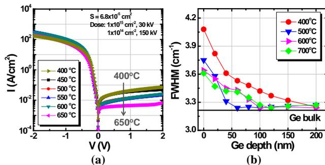
**Fig. 4** (a)  $I$ - $V$  characteristics of  $n^+/p$  junctions, where dopant activation was carried out at 400°C to 650°C. It shows good rectifying diode properties and much lower reverse current even annealed at 400°C, compared to Fig. 1(b). (b) Ge depth profile of FWHM in phosphorus implanted region after dopant activation annealing.
