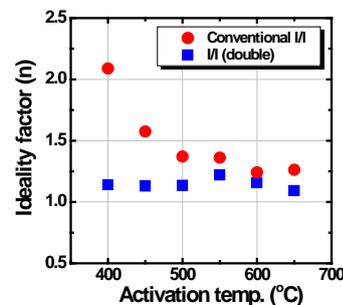
**Fig. 5** Ideality factor of  $n^+/p$  junction as a function of activation temperature. The value of  $n$  is a range of 1.1 to 1.2 for ion implantation with a double acceleration voltage and dose, regardless of the activation temperature.
