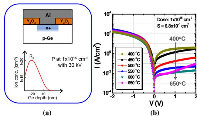
**Fig. 1** (a) Schematics of  $n^+/p$  diode and phosphorus concentration as a function of Ge depth. (b)  $I$ - $V$  characteristics of  $n^+/p$  junctions formed by a conventional ion implantation ( $1 \times 10^{15} \text{ cm}^{-2}$ , 30 kV), where dopant activation was carried out at 400°C to 650°C.
