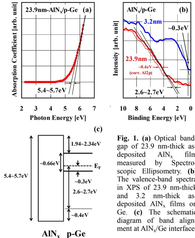
**Fig. 1.** (a) Optical band-gap of 23.9 nm-thick as-deposited AlN<sub>x</sub> film measured by Spectroscopic Ellipsometry. (b) The valence-band spectra in XPS of 23.9 nm-thick and 3.2 nm-thick as-deposited AlN<sub>x</sub> films on Ge. (c) The schematic diagram of band alignment at AlN<sub>x</sub>/Ge interface.
