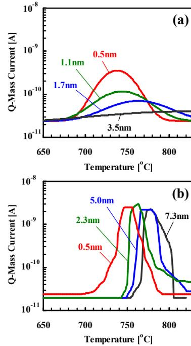
**Fig. 3.** The deconvoluted signals in the TDS spectra of the  $N_2$  desorption form  $AlN_x/10$  nm-thick  $GeN_x/Ge$  with  $AlN_x$  thickness dependence, including (a) the tail region given by the Gaussian function and (b) the sharp peak with threshold temperature given as the residual part after the Gaussian fitting.
