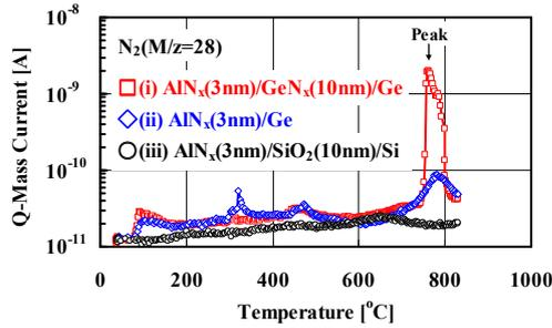
**Fig. 2.** TDS spectra of the  $N_2$  desorption form (i) 3 nm-thick  $AlN_x/10$  nm-thick  $GeN_x/Ge$ , (ii) 3 nm-thick  $AlN_x/Ge$ , and (iii) 3 nm-thick  $AlN_x/10$  nm-thick  $SiO_2/Si$  stacks. The heating was performed from room-temperature to  $830^\circ C$  with  $20^\circ C/min$ . Mass number 28 was selected for the detection of  $N_2$  desorpted from the samples.
