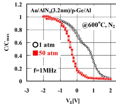
**Fig. 4.** The 1MHz bi-directional C-V characteristics of Au/3.2 nm-thick  $AlN_x/p-Ge(100)/Al$  MIS capacitors fabricated by the annealing of 1 atm and 50 atm  $N_2$ , processed at  $600^\circ C$ .
