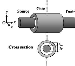
Fig. 1. NW MOSFET structure.
