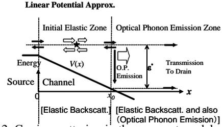
Fig. 2. Carrier scattering in the compact model of the quasi-ballistic NW MOSFET.
