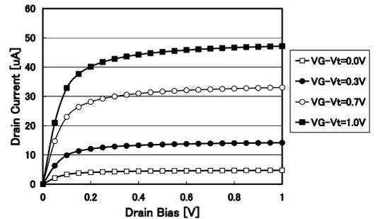
Fig. 8.  $I-V_D$  plot by the second formula in Fig. 5. The Boltzmann statistics model.
