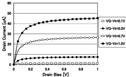
Fig. 7.  $I-V_D$  plot by the first formula in Fig. 4. The fully degenerate carrier model.
