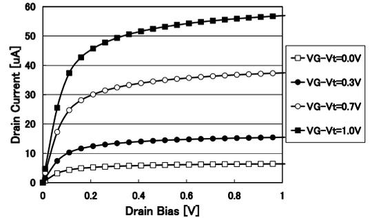
Fig. 6.  $I-V_D$  plot by the quasi-ballistic compact model previously proposed.
