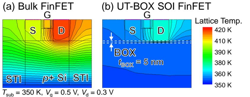
**Fig. 6:** Contour plots of lattice temperature ( $T_L$ ) for (a) Bulk and (b) UT-BOX SOI FinFETs under analog operation ( $V_g = 0.5 \text{ V}$  and  $V_d = 0.3 \text{ V}$ ). Even under the practical bias conditions for analog operation, the impact of SHE is prominent;  $T_L$  of Bulk FinFETs is higher than that of UT-BOX SOI FinFETs.
