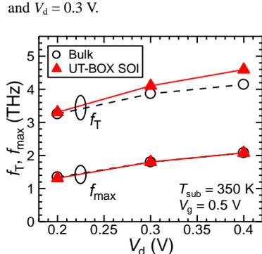
**Fig. 7:** Cutoff frequency ( $f_T$ ) and maximum oscillation frequency ( $f_{max}$ ) vs  $V_d$ .  $f_T$  of UT-BOX SOI FinFETs is higher than that of Bulk FinFETs. As  $V_d$  increases,  $f_T/f_{max}$  and  $f_T$  difference between Bulk and UT-BOX SOI FinFETs slightly increase.
