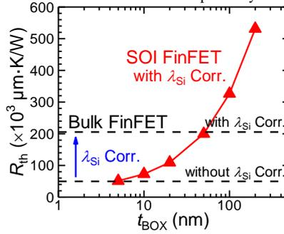
**Fig. 3:**  $R_{th}$  of SOI FinFETs (triangles) vs BOX thickness ( $t_{BOX}$ ) with  $\lambda_{Si}$  corrections (Fig. 2) and  $R_{th}$  of Bulk FinFETs (dashed lines) with and without  $\lambda_{Si}$  corrections. By taking into account the  $\lambda_{Si}$  corrections, it is shown that SOI FinFETs have thermal advantage when  $t_{BOX}$  is relatively thick ( $< 50 \text{ nm}$ ).
