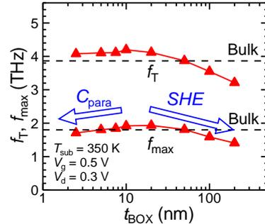
**Fig. 8:**  $f_T/f_{max}$  of SOI FinFETs (triangles) vs  $t_{BOX}$ .  $f_T/f_{max}$  of Bulk FinFETs are also shown (dashed lines).  $f_T/f_{max}$  of SOI FinFETs marked the peak around  $t_{BOX} = 10 \text{ nm}$ . This is because parasitic capacitance ( $C_{para}$ ) degrades  $f_T/f_{max}$  at the extremely thin BOX of 5 nm, whereas thick BOX increases device temperature and degrades transconductance.
