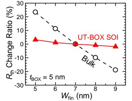
**Fig. 4:**  $R_{th}$  change ratio vs  $W_{fin}$  of Bulk and ultrathin-BOX (UT-BOX) SOI FinFETs. Although the variation in  $W_{fin}$  ( $\delta W_{fin}$ ) strongly affects  $R_{th}$  of Bulk FinFETs,  $R_{th}$  of SOI FinFETs is almost independent of  $\delta W_{fin}$ .
