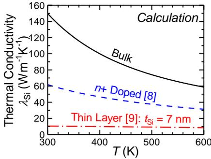
**Fig. 2:** Thermal conductivity ( $\lambda_{Si}$ ) of bulk,  $n+$  doped (phosphorus  $1.7 \times 10^{20} \text{ cm}^{-3}$ ) Si, and 7-nm Si slab as a function of temperature. This figure clearly shows that the conventional bulk  $\lambda_{Si}$  of  $148 \text{ Wm}^{-1}\text{K}^{-1}$  should be corrected for the  $R_{th}$  calculation. In heavily doped or thin Si,  $\lambda_{Si}$  degrades significantly due to decreased phonon mean free path.
