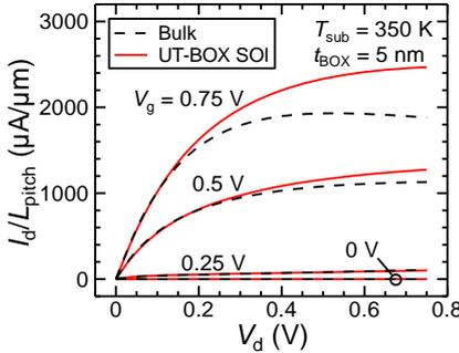
**Fig. 5:** Drain current divided by fin pitch ( $I_d/L_{pitch}$ ) vs drain voltage ( $V_d$ ). At higher gate voltage ( $V_g$ ) and  $V_d$  region,  $I_d/L_{pitch}$  of Bulk FinFETs is considerably lower than that of UT-BOX SOI FinFETs due to self-heating effect (SHE). The bias point for analog operations is set to be around  $V_g = 0.5 \text{ V}$  and  $V_d = 0.3 \text{ V}$ .
