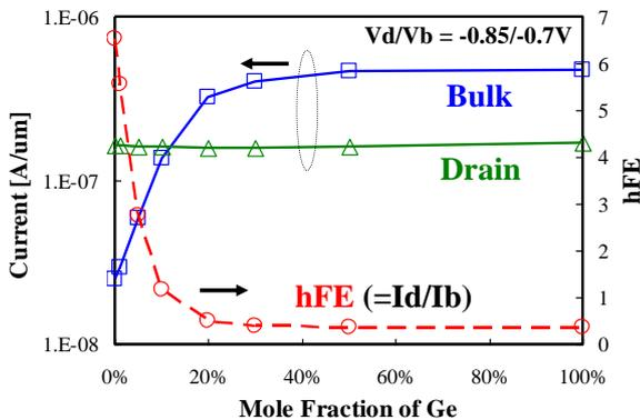
Fig. 5 Ge mole fraction dependences of drain, bulk currents and hFE in Si/eSiGe PMOS.
