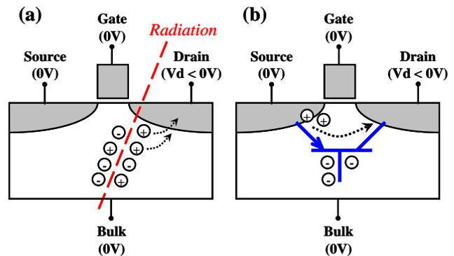
Fig. 1 Illustration of the parasitic bipolar effect in PMOS.
