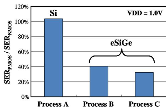
Fig. 3 The ratio between NMOS and PMOS SERs.
