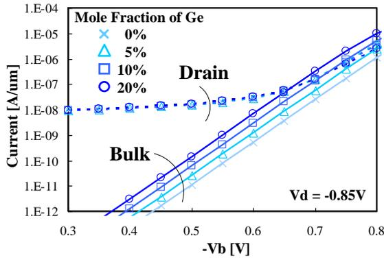
Fig. 4 Bulk bias voltage dependences of drain and bulk currents in Si/eSiGe PMOS.
