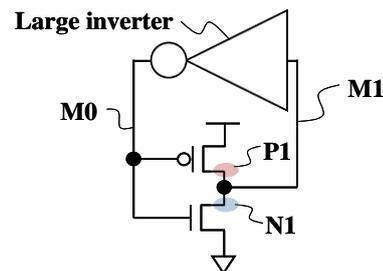
Fig. 2 Schematic of the unbalanced feedback-loop circuit.
