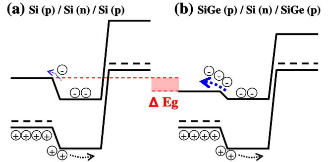
Fig. 6 Schematic band diagram of the parasitic bipolar transistor in Si/eSiGe PMOS.
