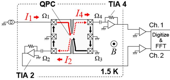
Fig. 2 Schematic setup of the cross-correlation measurement.
