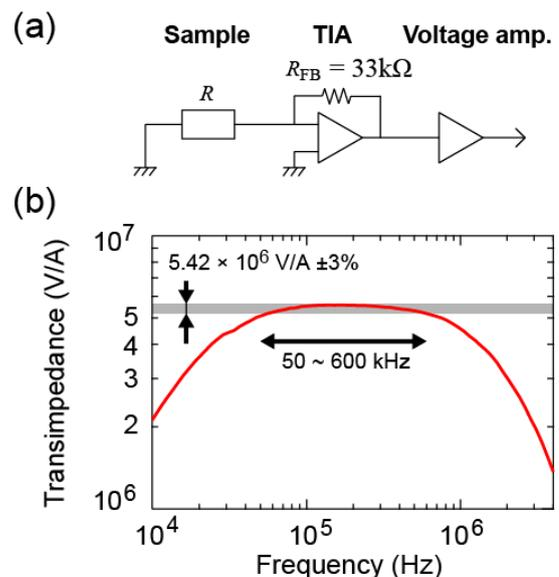
Fig. 1 (a) Schematic of the noise measurement system. (b) Frequency dependence of the transimpedance of the system shown in (a).
