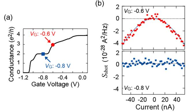
Fig. 3 (a) Conductance of the QPC as a function of the gate voltage. (b) Shot noise as a function of the current  $I_1$ . We observed negative  $S_{\text{shot}}$  at  $V_G = -0.6$  V (upper panel), while no shot noise at  $V_G = -0.8$  V (lower panel).
