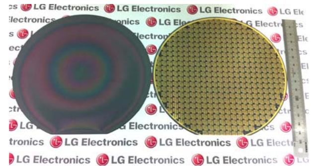
Fig 5. Top view image of crack-free-6um-thick GaN on 6-inch Si substrate and fully processed wafer
