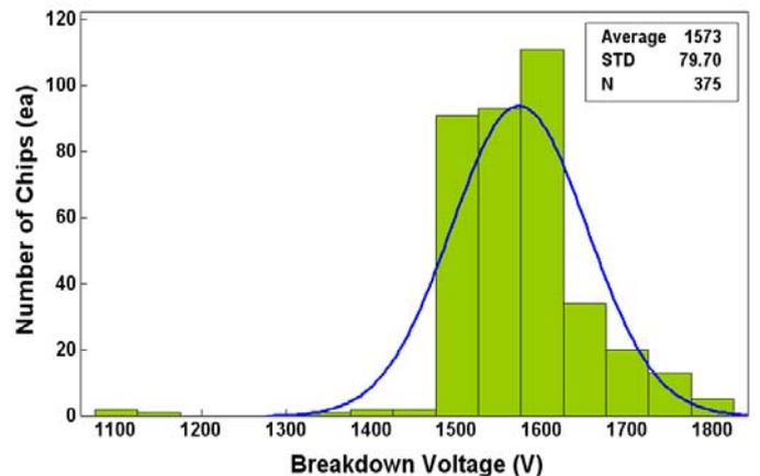
Fig 7. Histogram of breakdown voltage from 6-inch wafer
