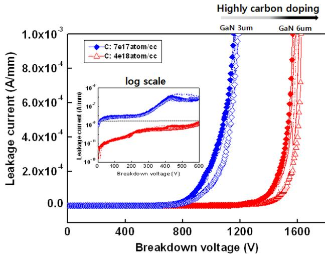
Fig 3. Leakage reduction with carbon concentration and GaN thickness
