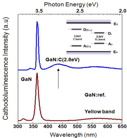
Fig 2. Low-temp. (77K) cathodoluminescence spectra of carbon-doped GaN(top) and UID-GaN(bottom)
