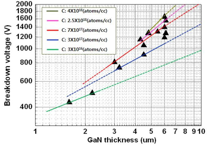
Fig 4. Breakdown voltage with carbon concentration and GaN thickness
