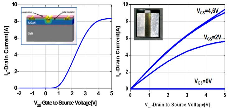
Fig 6. (a) Normally-off characteristic ( $V_{th}=0.7V$ ) of HFET device (b) Output  $I_d$ - $V_d$  characteristics ( $I_d=5A$ ) of HFET device
