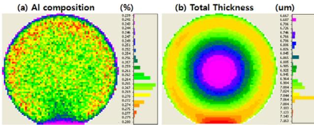
Fig 1. PL Mapping of (a) the Al composition and (b) thickness
