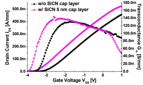
Fig. 2(a). Transfer characteristics and transconductance curve of the fabricated Schottky HEMT ( $V_{DS} = 10$  V)
