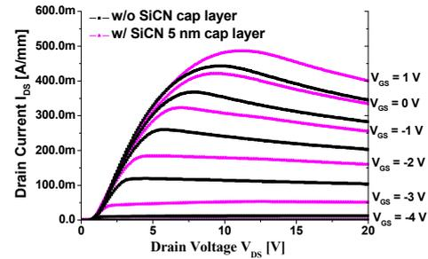
Fig. 3. Family curve of fabricated Schottky-drain HEMT
