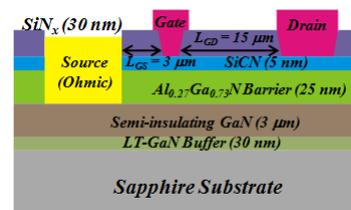
Fig. 1. Schematic sketch of the fabricated SiCN-HEMT
