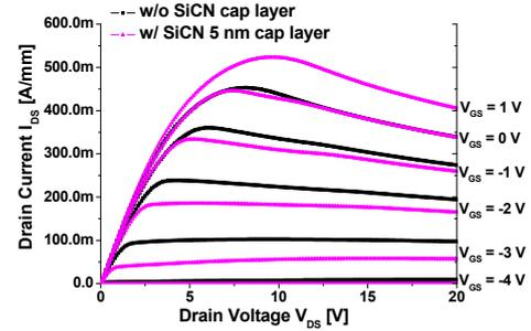
Fig. 2(b). Family curve of fabricated Schottky HEMT
