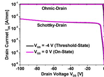
Fig. 4. Reverse blocking capability due to the integrated protection diode
