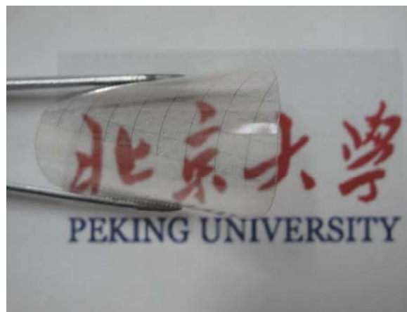
Fig. 2 Image of transparent AZO thin-film transistor on a bent flexible PET substrate
