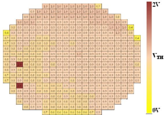
Fig. 6 The mapping data of  $V_{TH}$  characteristics of HFETs on 6-inch Si substrate
