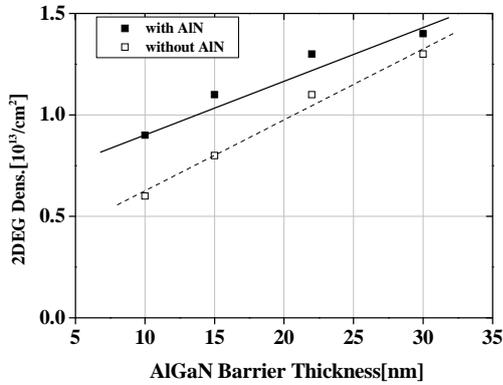
Fig. 3 2DEG density as a function of AlGaN barrier thickness
