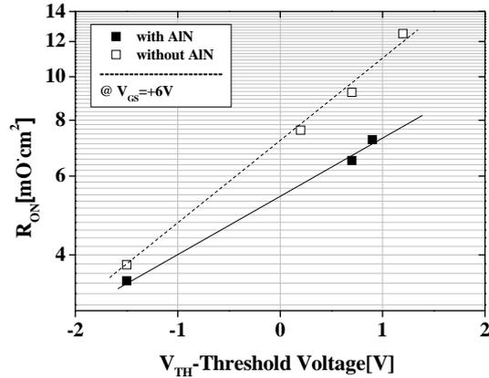
Fig. 7 Specific on-state resistance versus threshold voltage for normally-off p-GaN/AlGaN/GaN HFETs with and without AlN interlayer
