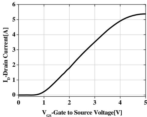
Fig. 4 Transfer characteristic for 24mm wide devices with  $L_{GD}=15\mu m$  on a 6-inch Si substrate.  $V_{DS}=5V$
