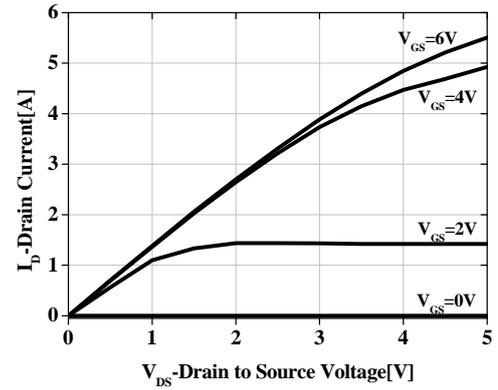
Fig. 5 Output characteristic for 24mm wide devices with  $L_{GD}=15\mu m$  on a 6-inch Si substrate.
