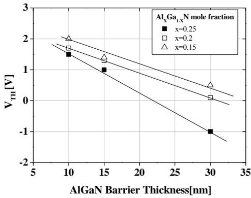
Fig. 2 Threshold voltage characteristics for changing Al mole fraction and thickness of AlGaN barrier
