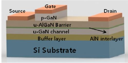
Fig. 1 Schematic cross-sectional view of p-GaN gate HFET
