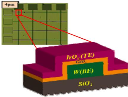
Fig. 1 Optical image and schematic view of the crossbar resistive switching memory devices using IrO<sub>x</sub>/GdO<sub>x</sub>/W structure are shown. The device size is 4x4 μm<sup>2</sup>.
