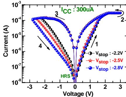
Fig. 8 I-V hysteresis loop with the variation of stop voltage of our IrO<sub>x</sub>/GdO<sub>x</sub>/W crossbar memory device. The HRS increases with increasing the negative voltages.
