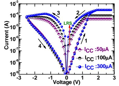
Fig. 6 I-V hysteresis loop of IrO<sub>x</sub>/GdO<sub>x</sub>/W crossbar memory device with the variation of I<sub>CC</sub> from 50-300 μA. Multi-level data storage is observed.
