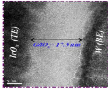
Fig. 2 Cross-sectional HRTEM image of IrO<sub>x</sub>/GdO<sub>x</sub>/W crossbar memory device. Thickness of GdO<sub>x</sub> layer is ~ 17.5 nm.
