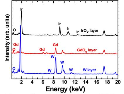
Fig. 3 Energy dispersive X-ray spectra (EDX) shows Ir, Gd, W, and O elements from Fig. 2. It proves layer-by-layer structure with presence of GdO<sub>x</sub> resistive switching layer.
