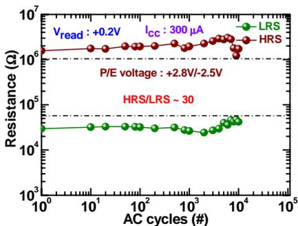
Fig.10 Excellent AC endurance of >10<sup>4</sup> cycles of our IrO<sub>x</sub>/GdO<sub>x</sub>/W memory device. The resistance states were read out at +0.2V.
