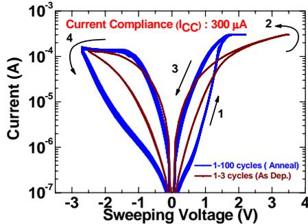
Fig. 4 Repeatable typical I-V hysteresis loop of our IrO<sub>x</sub>/GdO<sub>x</sub>/W crossbar memory device is observed after annealing. A low operation voltage of < ±3V is applied to achieve repeatable and reproducible cycles.
