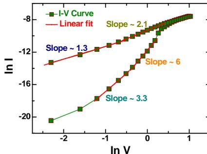
Fig. 5 I-V curve are re-plotted in log-log scale. Both resistance state exhibits trap controlled space charge limited current conduction mechanism.
