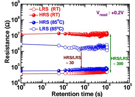
Fig. 12 Excellent retention characteristics of >10<sup>4</sup> s at RT and 85°C of our IrO<sub>x</sub>/GdO<sub>x</sub>/W crossbar memory device are reported.
