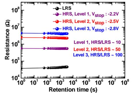
Fig. 9 Excellent multilevel retention characteristics with the variation of stop voltage of our IrO<sub>x</sub>/GdO<sub>x</sub>/W crossbar memory device are observed.
