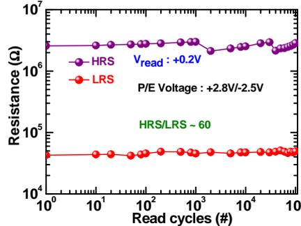
Fig.11 Good read cycles of 10<sup>5</sup> cycles of our crossbar memory device. Both resistance states were read out at +0.2V.
