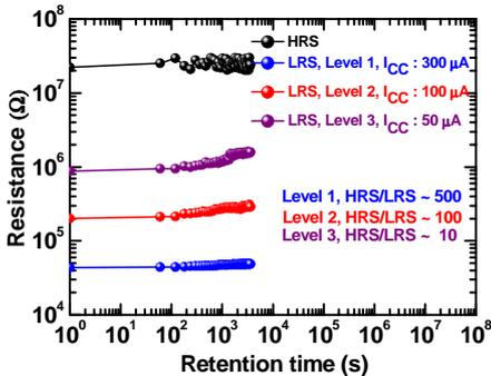
Fig. 7 Excellent multilevel retention characteristics of IrO<sub>x</sub>/GdO<sub>x</sub>/W crossbar memory device with different current compliances.
