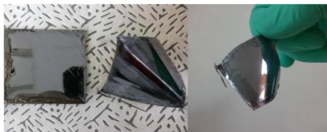
Fig. 5 Pictures of 3.5x3.5 cm<sup>2</sup> ~50μm thin Si film along with the residual wafer after lift-off.
