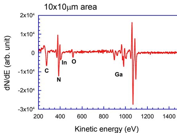
Fig. 2: AES chart of step-free InN ultrathin layer formed on step-free GaN surface.
