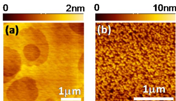
Fig.3: AFM images of (a) partially coalesced 2D islands of InN formed on a step-free GaN surface using  $t_D$  of 5 s at 530 °C and (b) 3D dots of InN formed using  $t_D$  of 10 s at 530 °C.
