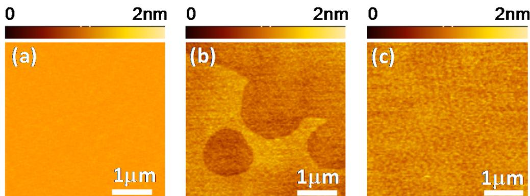
Fig.1: AFM images of (a) step-free GaN surface formed within a hexagonal-shaped selective-area having no screw-type dislocations, (b) partially coalesced 2D islands of InN formed on a step-free GaN surface using  $t_D$  of 10 s at 620 °C, and (c) step-free InN surface formed using  $t_D$  of 30 s at 620 °C.
