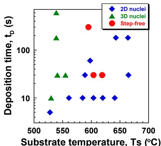
Fig.4: Morphologies of InN layers plotted as functions of  $t_D$  and  $T_s$ . Closed diamonds, triangles, and circles correspond to 2D nuclei, 3D nuclei, and step-free surfaces of InN, respectively.
