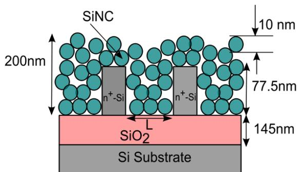
Fig. 1 Schematic diagram of device structure (cross-section view). Channel length  $L$  is varied between 20-200 nm.
