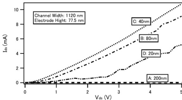
Fig. 4  $I$ - $V$  characteristics for device with  $L = 200\text{nm}$ ,  $80\text{nm}$ ,  $40\text{nm}$  and  $20\text{nm}$ .
