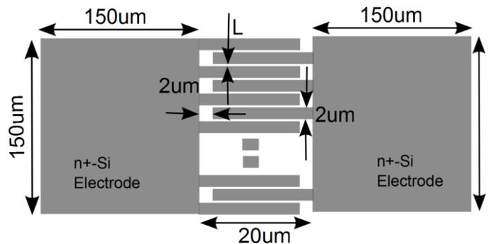
Fig. 2 Schematic diagram of inter-digital electrode (top view).
