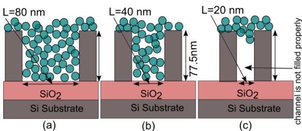
Fig. 5 Schematic model of devices with different channel length  $L$
