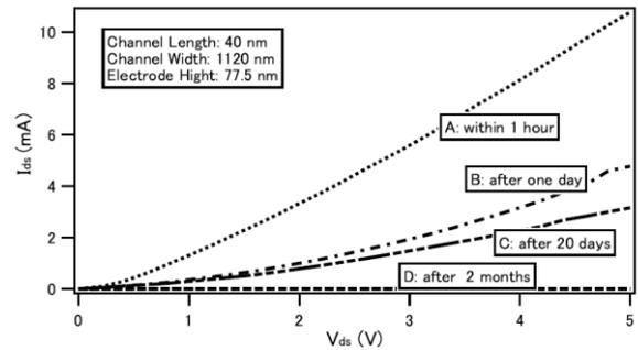
Fig. 6 Time dependent  $I$ - $V$  characteristics for device with  $L = 40\text{nm}$ .
