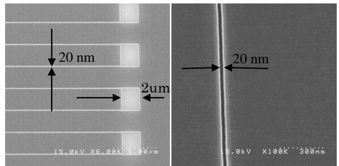
Fig. 3 SEM image of inter-digital electrode (top view) for device with  $L = 20$  nm. Dark area is Si, white area is gap (left). Magnified view of the electrode gap of 20 nm (right).
