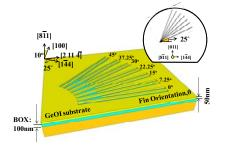
Fig. 1. Fins with different orientations ( $\theta = 0^{\circ}$  to 45°) are defined on a 10° Offcut GeOI substrate.
