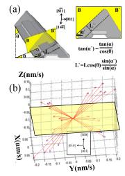
Fig. 6. (a) Method to extract growth rate in a direction perpendicular to facet plane. Growth rate is proportional to L'. (b) Growth rate of GaAs in various crystal orientations. The ratio of growth rates of  $\{811\}:\{111\}A:\{110\}:\{111\}B$  is measured to be 19:8:11:2.
