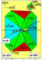
Fig. 4. Equilibrium Crystal Shape (ECS) showing the facets formed when growth is done on an infinitesimally small seed. The slow growing facets are {110}, {111}A and {111}B. ECS predicts the GaAs facets in our fin structures. Inset shows a tilted (10° offcut) ECS. Cut-plane through the ECS center perpendicular to the fin orientation  $\theta$  (mark by dotted lines) predicts the GaAs facets on the  $\theta$  oriented fin.
