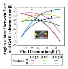
Fig. 5. Angles  $\alpha$  and  $\beta$  subtended between facet faces and GeOI {811} surface as a function of fin orientation. Measured angles from TEM are plotted as solid symbols, and simulated angles are plotted as lines.
