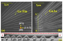
Fig. 2. SEM image of (a) Ge fins before growth and (b) GaAs on Ge fins after growth. (c) TEM cross section along A-A' shows a faceted growth of GaAs on Ge fin.
