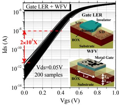
Fig. 4. The distribution of  $I_{ds}$ - $V_{gs}$  characteristics of UTB SOI MOSFET considering gate LER and WFV.
