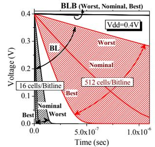
Fig. 8. The BL/BLB voltages with 16 and 512 cells per Bit-line at  $V_{dd}=0.4V$ .
