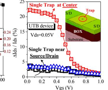
Fig. 12. Dependence of RTN amplitude on the position of trap at channel/gate insulator interface of UTB SOI device.
