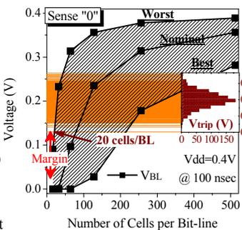
Fig. 10. Margin of large-signal inverter sense amplifier. The margin is defined by where all possible BL levels should be smaller than the minimum  $V_{trip}$ .
