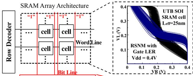
Fig. 1. Schematic of SRAM array in READ operation.
