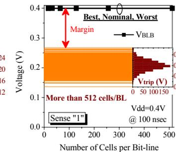
Fig. 11. Margin of large-signal inverter sense amplifier. The  $V_{trip}$  distribution should be lower than the possible BLB levels at the end of sensing action.
