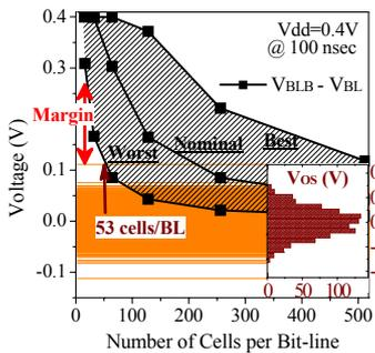
Fig. 9. Margin of differential CLSA at  $t=100$  nsec. The values of Bit-line differential voltage should be larger than the maximum of  $V_{OS}$  dispersion (orange lines) to ensure correct sensing action.
