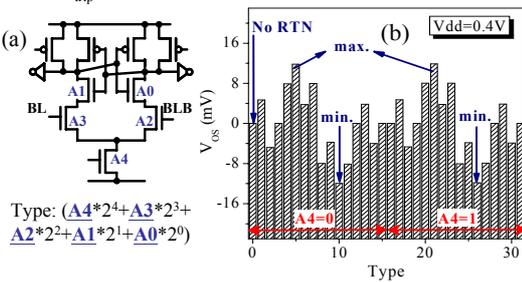
Fig. 14. (a) Binary-coded definition of trapping/de-trapping in each device for RTN analysis in CLSA and (b) the possible  $V_{OS}$  of various trapping/de-trapping combinations. (c) Comparison of  $V_{OS}$  distributions between the worst-case (max.  $V_{OS}$ ) combination and the case without RTN.
