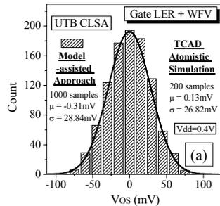
Fig. 6. (a) Comparison of  $V_{OS}$  variation between TCAD atomistic simulations and model-assisted approach considering gate LER and WFV and (b) the  $V_{OS}$  variation at various  $V_{dd}$ .
