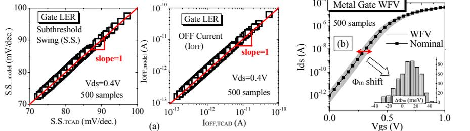
Fig. 5. Model calibration with atomistic TCAD simulations to build model libraries for gate LER and WFV. (a) The error analysis of S.S. and  $I_{OFF}$  for gate LER, and (b) determination of WFV library by  $\Phi_m$  ( $V_T$ ) shift.
