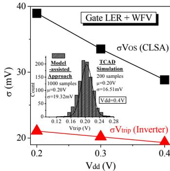
Fig. 7. Variability comparison of CLSA and inverter sense amplifier. The inset shows the  $V_{trip}$  comparison between TCAD simulation and model-assisted approach at  $V_{dd}=0.4V$ .
