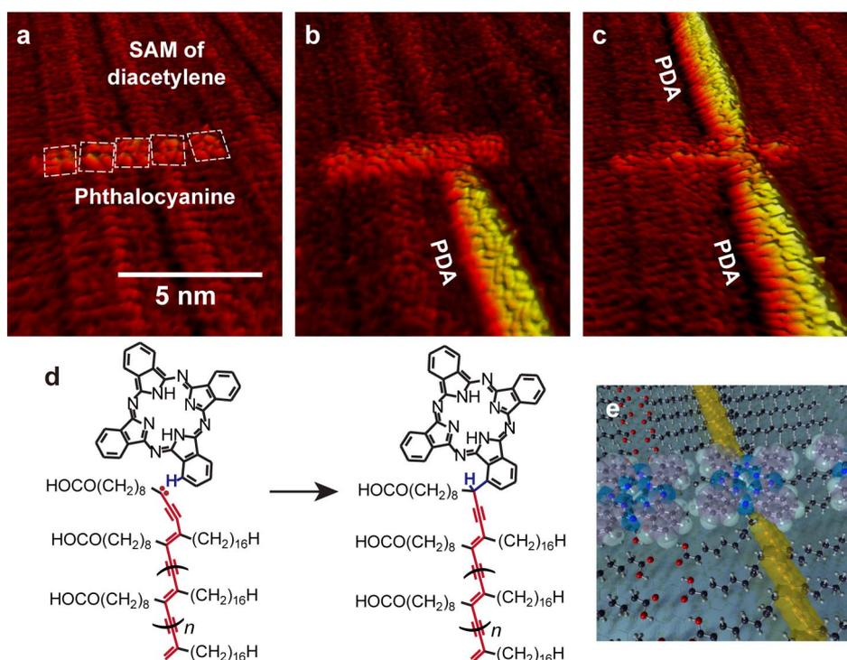
Fig. 3 (a-c) STM images showing the connection of two PDA chains to a single phthalocyanine molecule. (d) Proposed chemical reaction. The reactive end of PDA is inserted into a C-H bond of phthalocyanine. (e) Schematic structure model.
