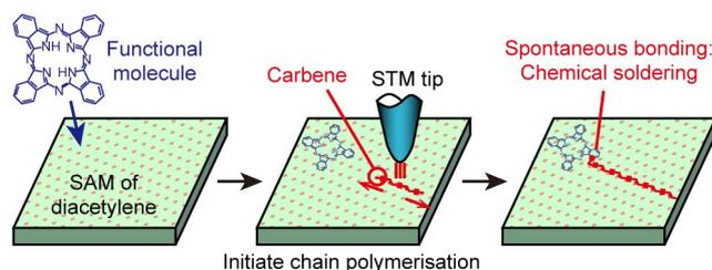
Fig. 2 Scheme of chemical soldering.
