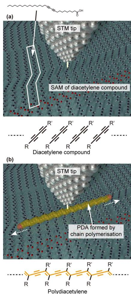
Fig. 1 (a) Chain polymerization of diacetylene compound is initiated by using an STM tip. (b) A single linear polydiacetylene chain can be created at any designated positions.
