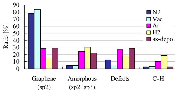
Fig. 3 Components of HAXPES C1s spectra in Co/C film after annealing at 800°C in various ambient gases
