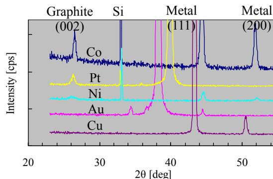
Fig. 2 XRD patterns ( $\theta$ -2 $\theta$ ) of carbon film with various catalyst layers after annealing at 800°C in N<sub>2</sub> flow gas
