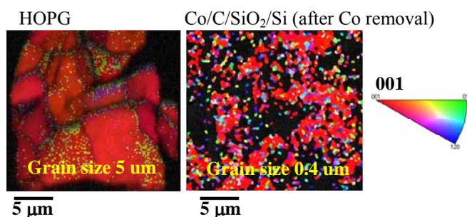
Fig. 6 EBSD of HOPG and Co/C film after Co removal
