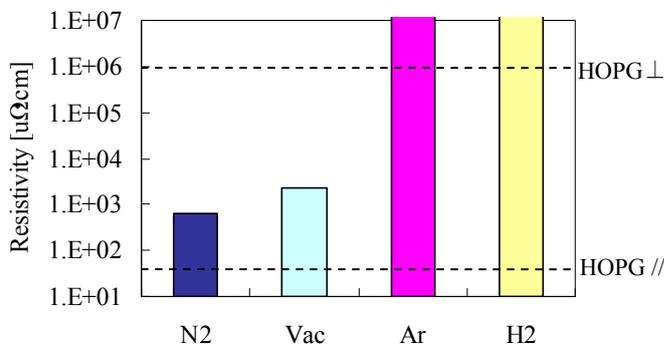
Fig. 5 Resistivity of a carbon film after removing Co of a Co/C film annealing at 800°C in various ambient gases
