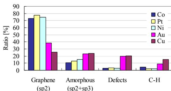
Fig. 1 Components of HAXPES C1s spectra in carbon film with various catalyst layers after annealing at 800°C in N<sub>2</sub> flow gas
