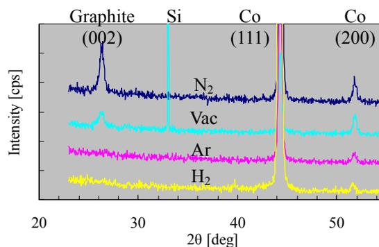
Fig. 4 XRD patterns (θ-2θ) of Co/C film after annealing at 800°C in various ambient gases
